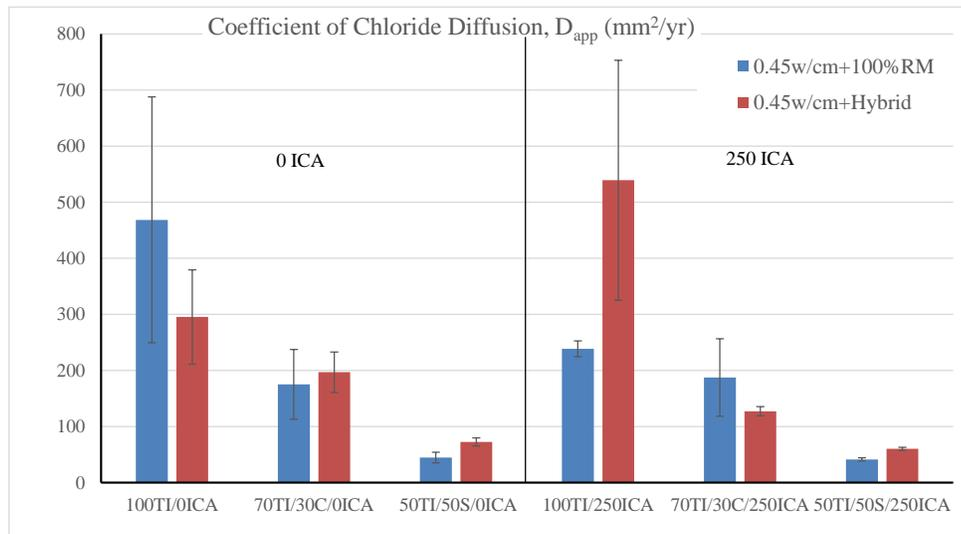
The apparent coefficient of chloride diffusion testing results are shown in Figure 5. The mixtures with w/cm of 0.45 had a much higher apparent coefficient of chloride diffusion than those with w/cm of 0.35, which matches the observation from surface resistivity testing. This is likely due to the higher porosity of the specimen with the higher water-to-cementitious
