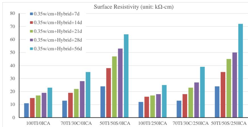
(b) Surface resistivity for 0.35 w/cm + 100% RH curing
