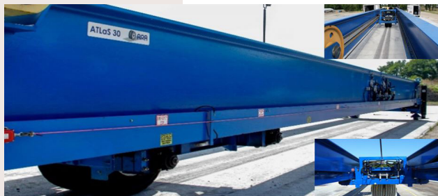
ATLaS30 is a heavy load simulation device located at LTRC's Pavement Research Facility, where pavement testing simulates 20 years of pavement trafficking in just a few months.
