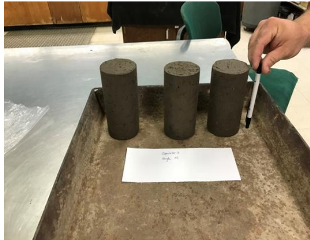
Figure 36. Samples prepared for UU test.
