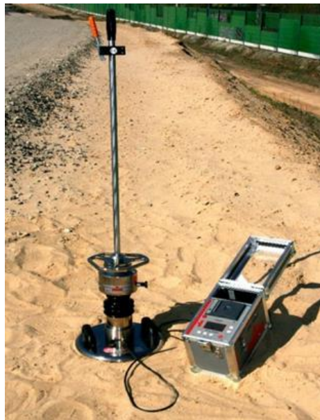
Figure 125. Light falling weight deflectometer
