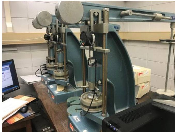
Figure 41. One-dimensional consolidation test
