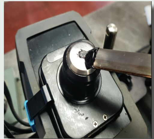
Figure 2. Placing sample on diamond ATR sensor of FT-IR
