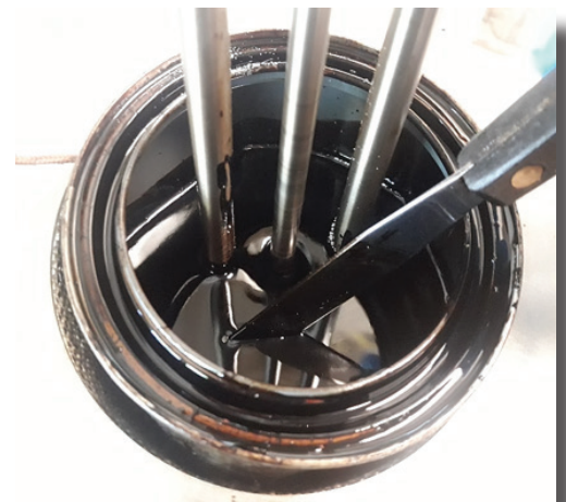
Figure 1. Sample collection technique for FT-IR spectroscopy
