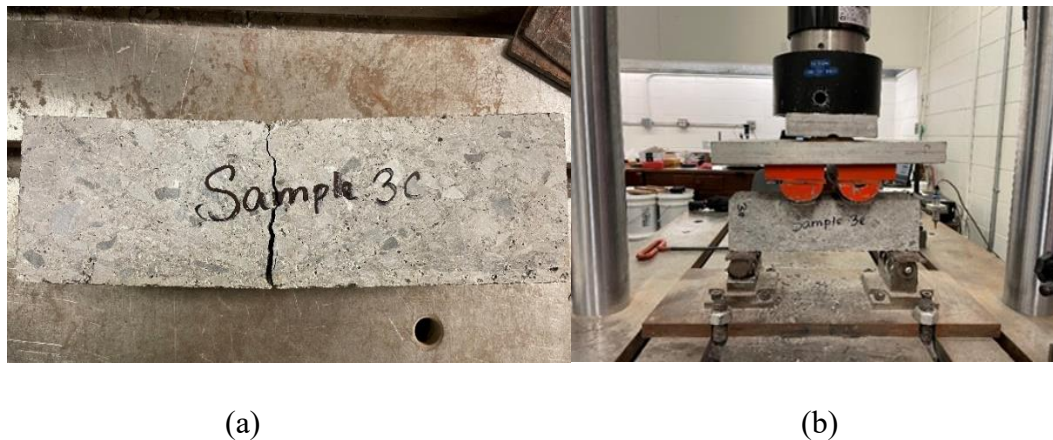
Figure 17. (a) Cracked specimen due to flexure (b) Cyclic loading at MTS (c) Failure of a specimen under cyclic loading (d) Obtained cycles to failure at SR = 0.9
