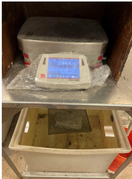
Figure 16. Density and specific gravity testing of RCC specimen
