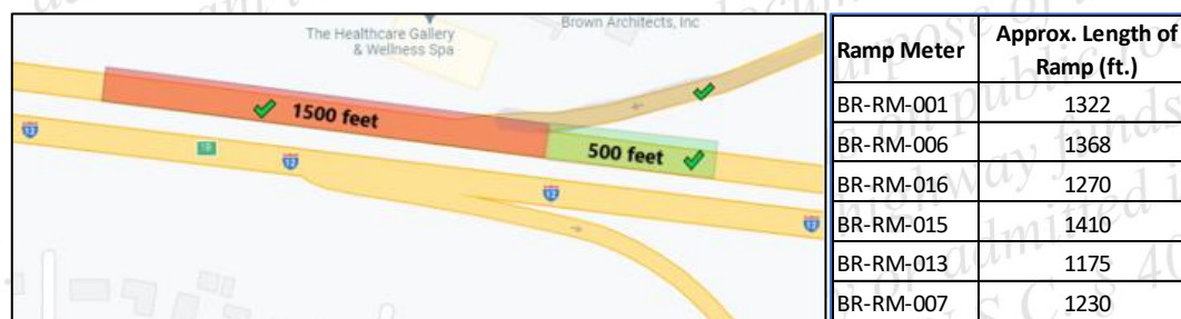
Figure 23. Data collection zones on a ramp meter
