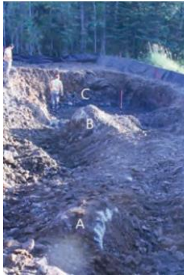
Figure 19. Photo of excavated site associating features with two high resistivity regions (A and B) and low resistivity region (C) in resistivity results (courtesy of MnDOT) [3]
