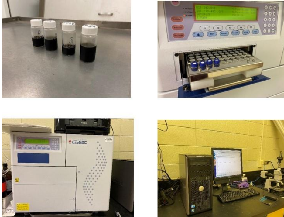
Figure 20. HP-GPC testing using EcoSEC HLC-8320GPC
