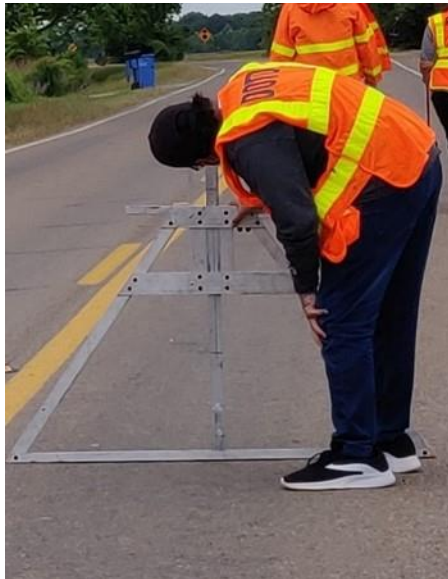
Figure 31. Rutting measurement along the wheel path
