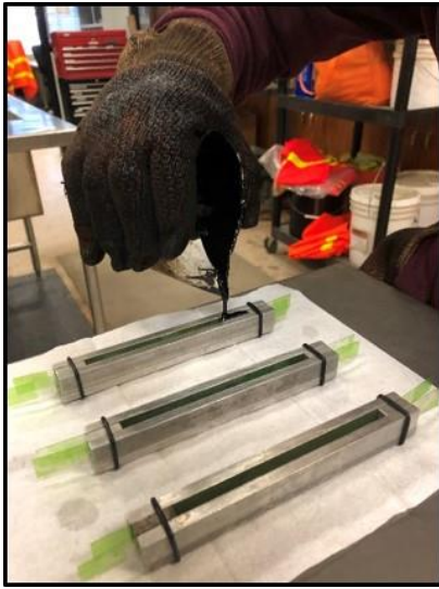
Figure 18. Bending Beam Rheometer (BBR) test; (a) mold preparation before testing (b) BBR machine
