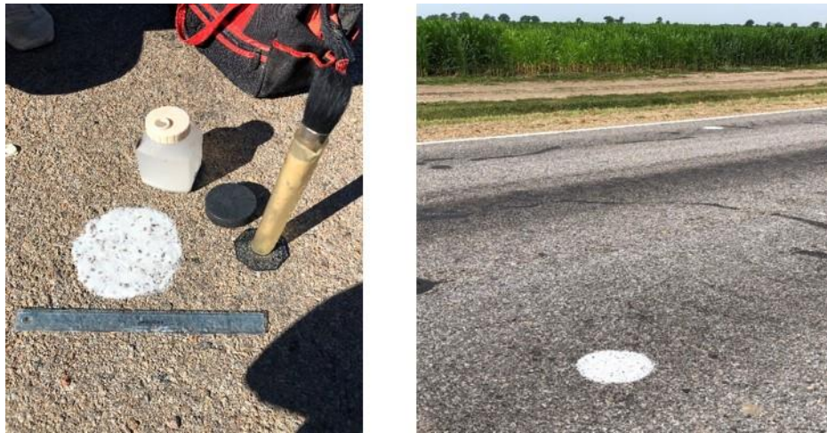
Figure 27. Sand patch test locations in CRS-2TR (0.37 gsy) and CRS-2TR (0.42 gsy)
