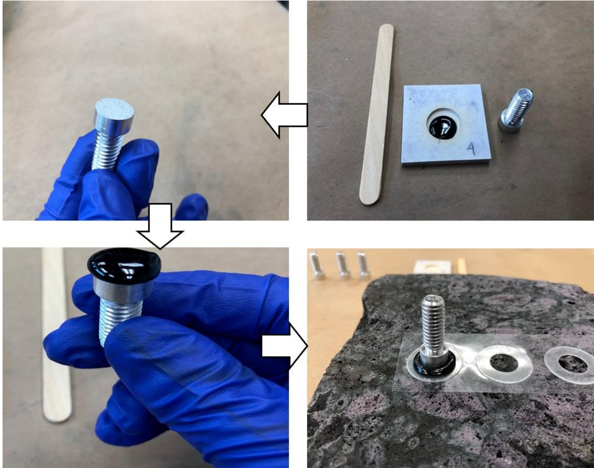
Figure 24. Preparation of bond strength test specimen
