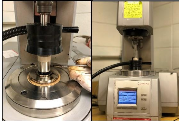
Figure 17. Dynamic Shear Rheometer (DSR) test; (a) sample trimming (b) DSR machine
