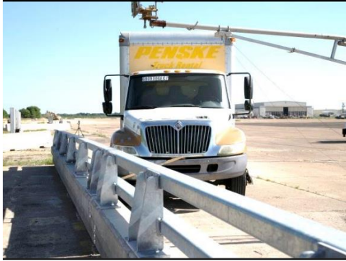
(a) 10000S test vehicle at impact point
