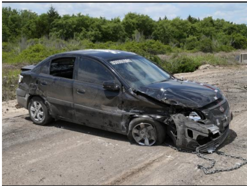
(a) Damage to right side
