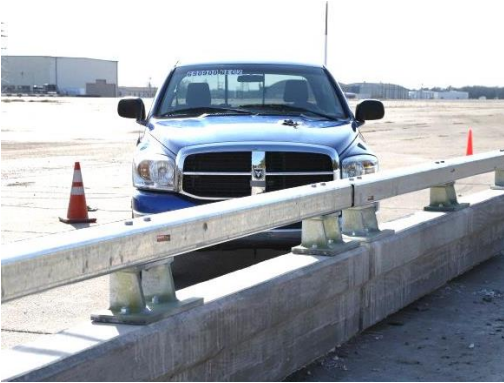
(a) Test vehicle at target impact point
