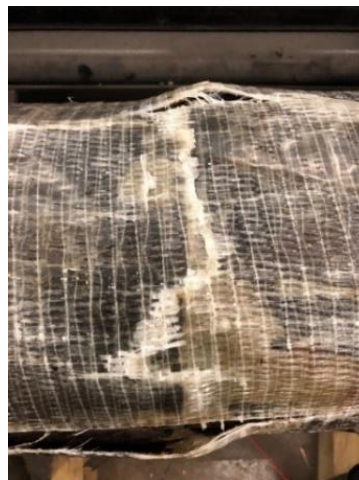
Figure 124. FRP splice cracking under applied load
