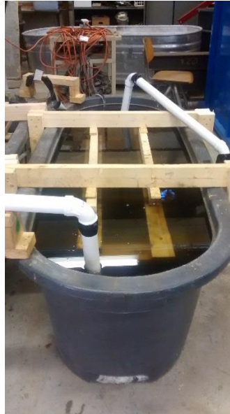
Figure 38. Saturated aging specimens
