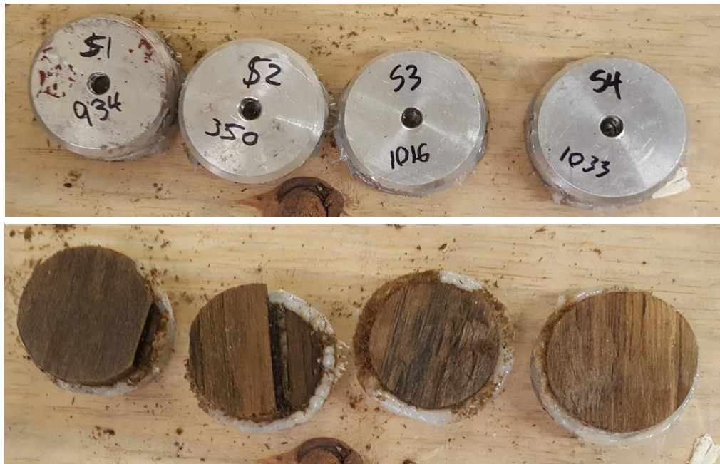
Figure 80. Sika pull-off carriers (timber failure)
