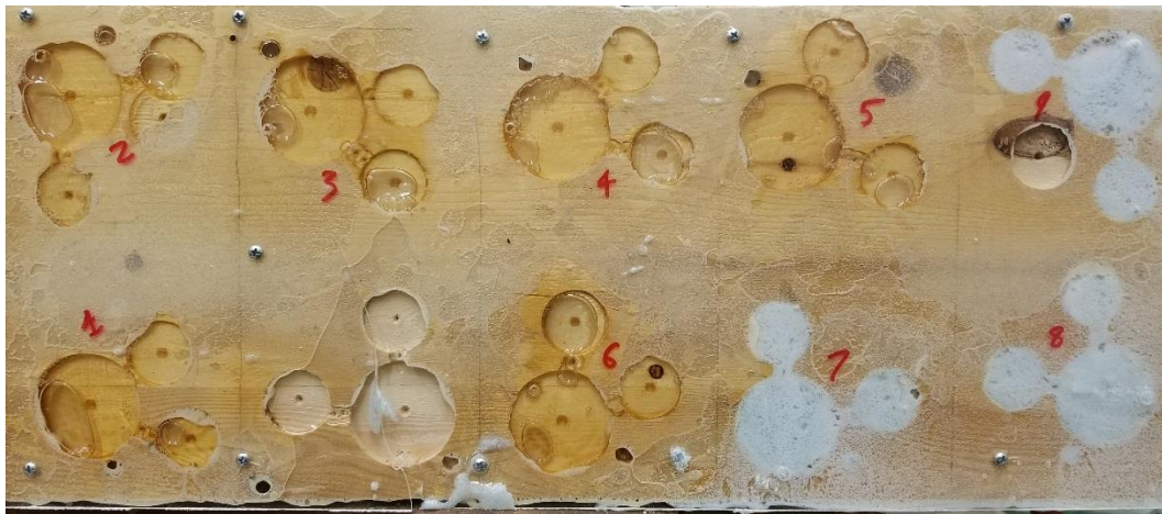
Figure 100. Large interconnected voids
