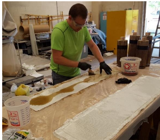
Figure 30. Apply resin to wraps for smaller mock up sample
