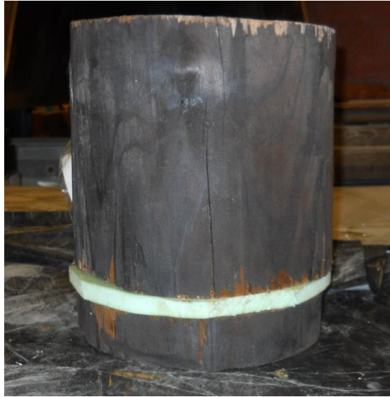
Figure 27. Unwrapped timber bond specimen
