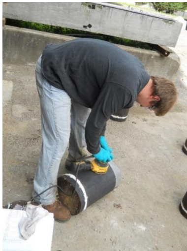
Figure 28. Sanding of bond specimens
