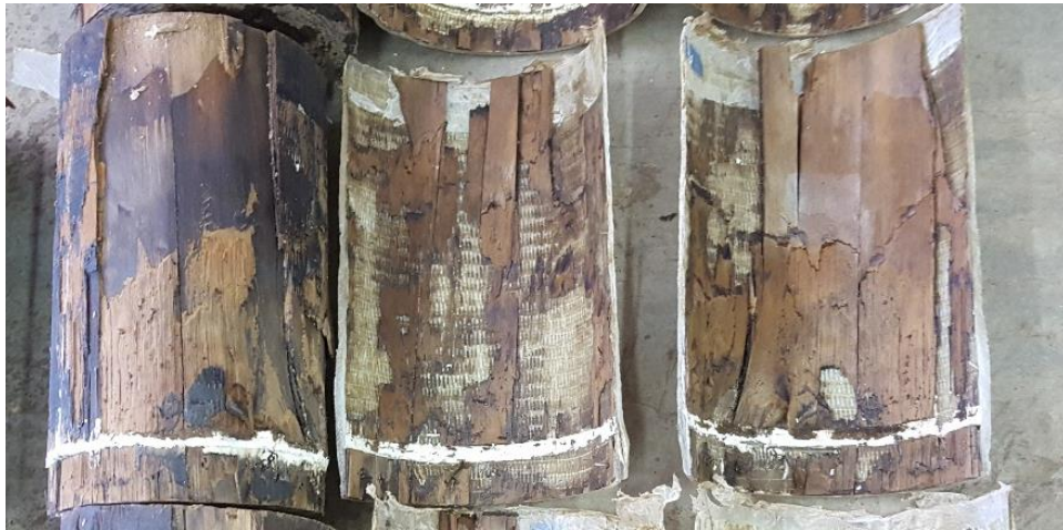
Figure 68. Retained timber on Fyfe bond tests
