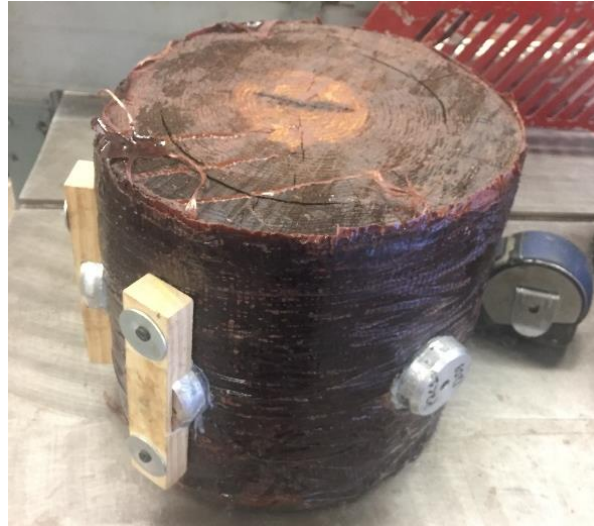
Figure 40. Pull-off puck attachment technique
