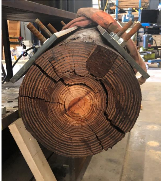
Figure 120. Cracking of steel splice pile at contact surface
