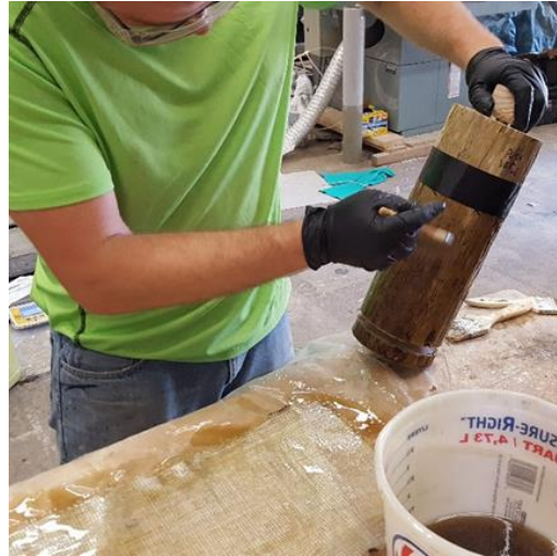
Figure 29. Apply primer to smaller mock up sample
