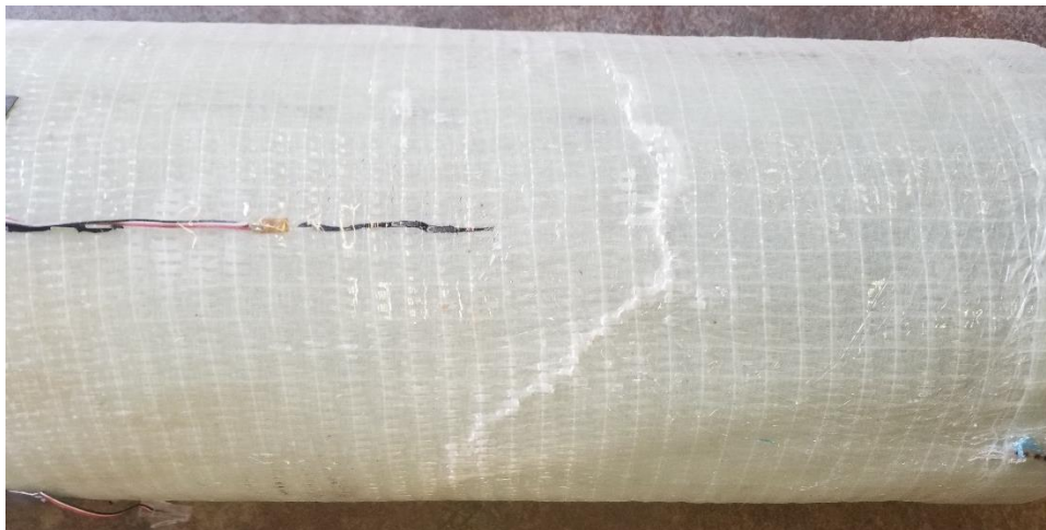
Figure 96. Failure of combined axial and bending
