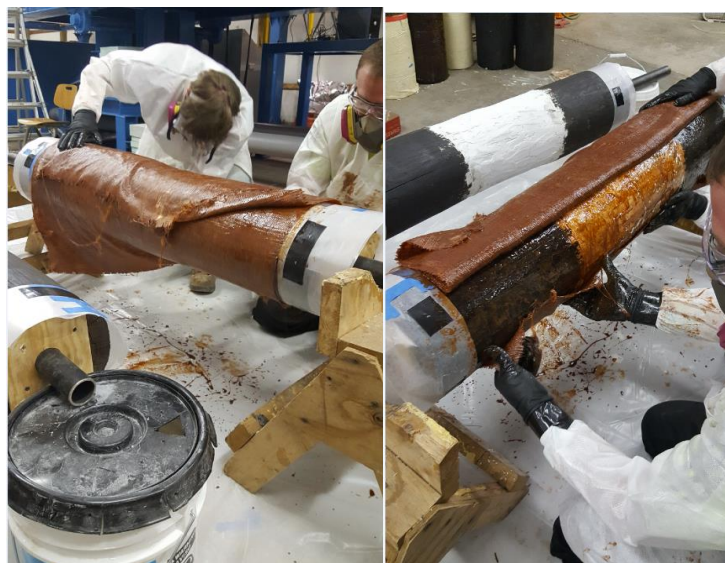
Figure 50. Wrapping of rehabilitation specimens
