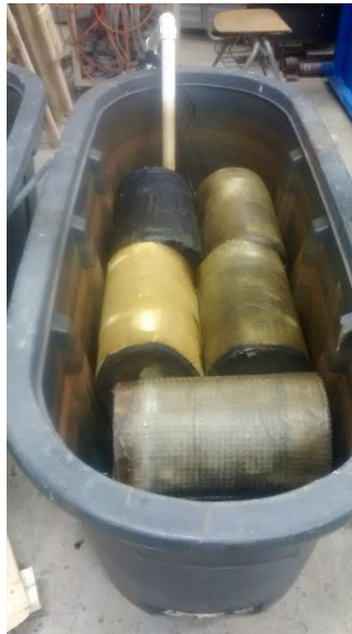
Figure 37. Aging specimens in tanks
