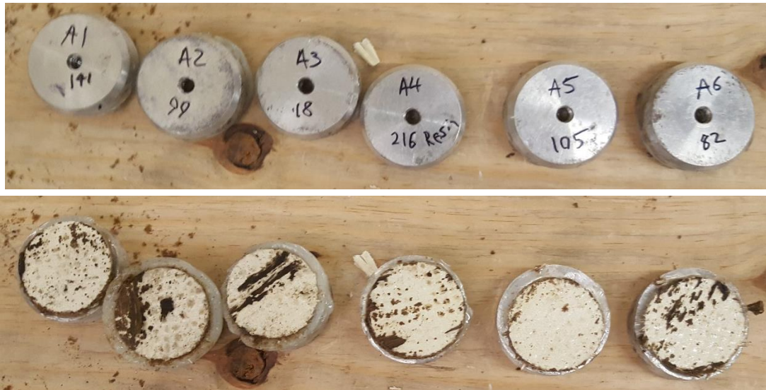
Figure 83. Aquawrap pull-off carriers (bond line)
