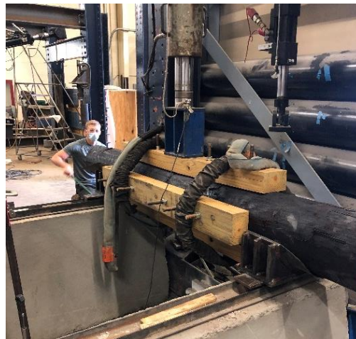
Figure 63. Shear test setup with wooden splice
