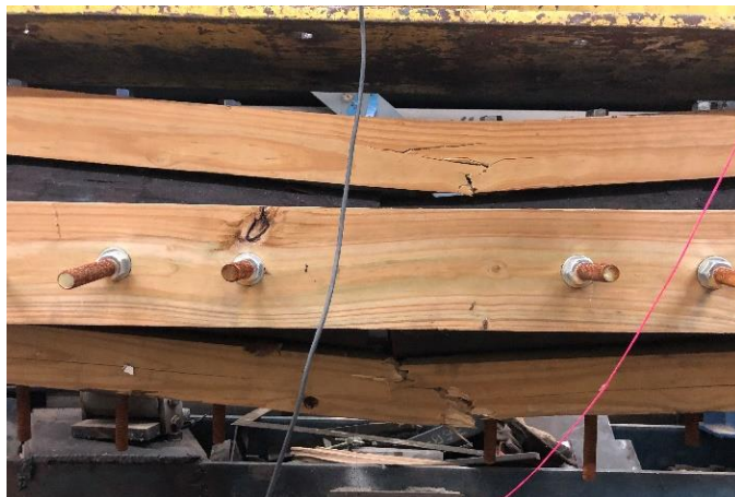
Figure 116. Wood splicing crack during flexure test
