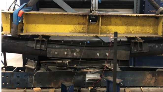
Figure 114. Steel splice yielding during bending test
