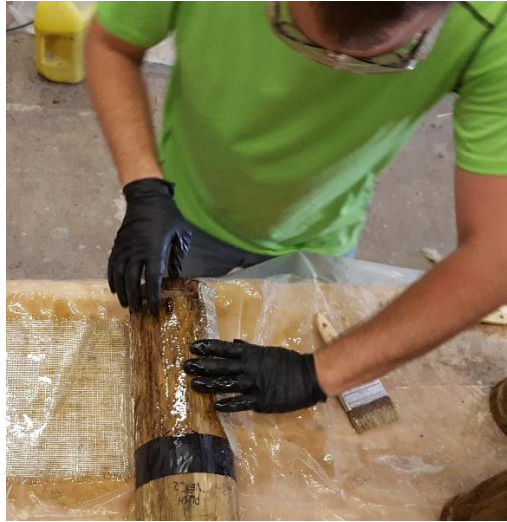
Figure 32. Wrapping smaller mock sample
