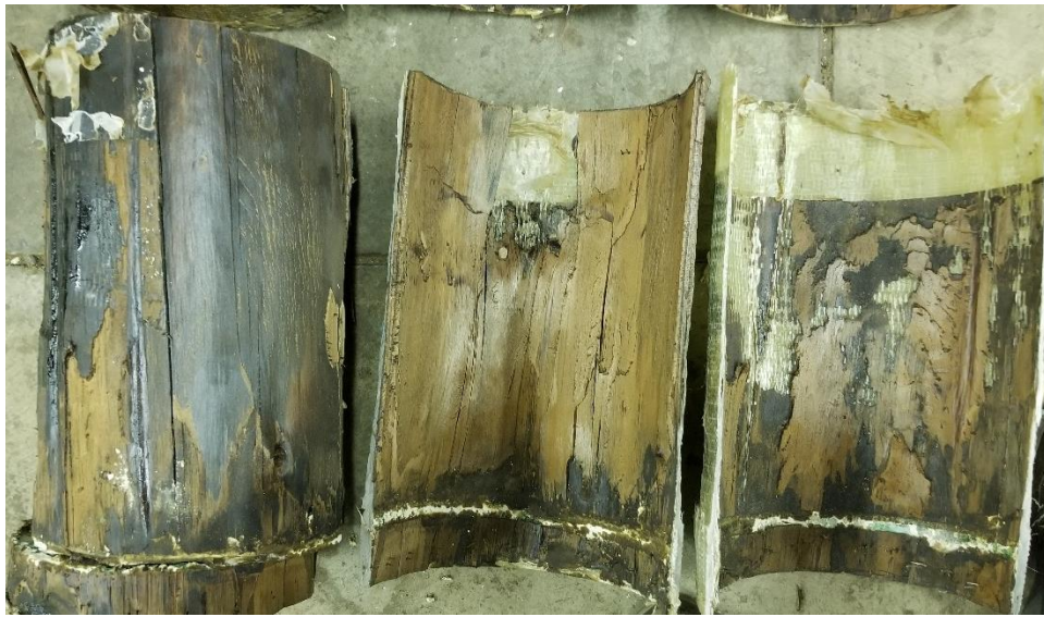
Figure 72. Retained timber on Simpson Strong Tie bond test
