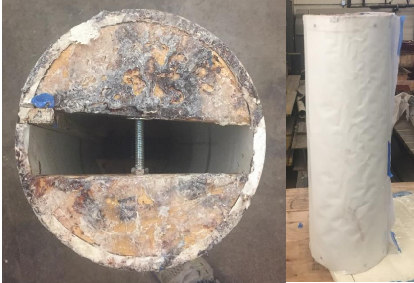
Figure 42. PVC mold for compression testing
