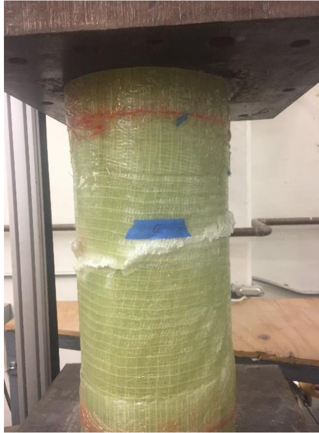
Figure 84. Typical Fyfe compression failure (Fyfe E)
