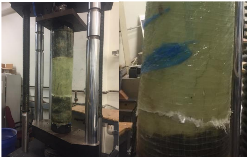
Figure 95. Typical simulated rehab failure
