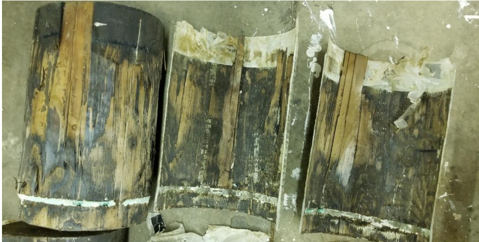
Figure 70. Retained timber on Sika bond tests
