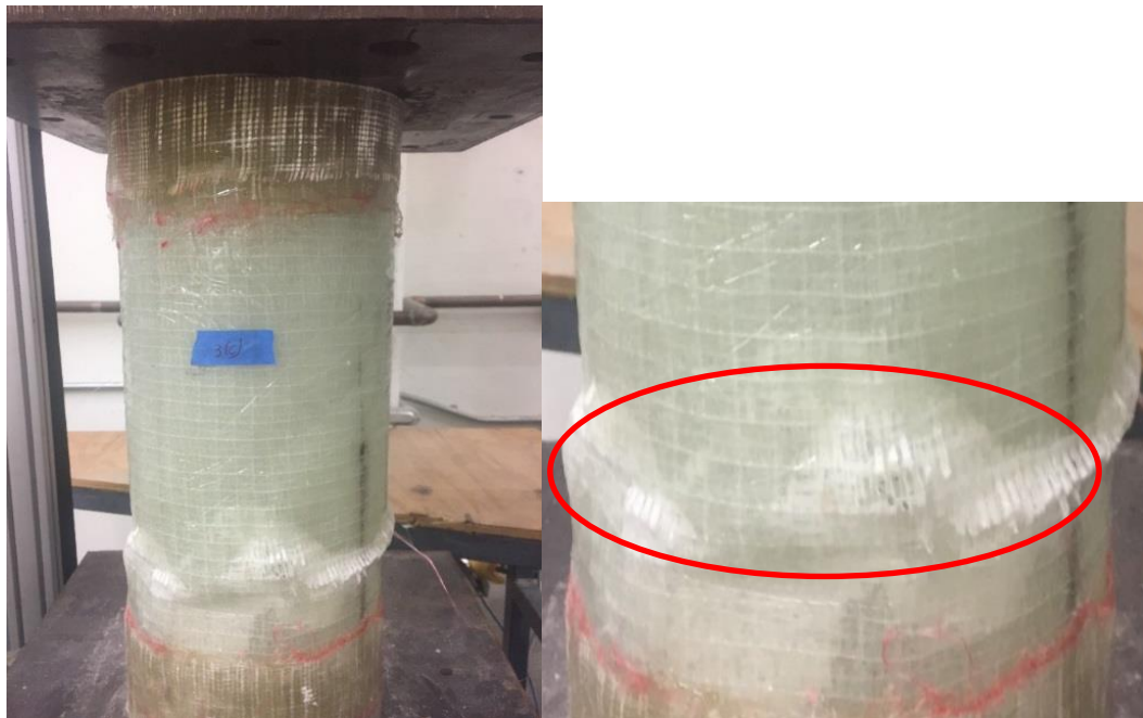
Figure 86. Typical compressive failure of sika system (Sika C) in the fibers
