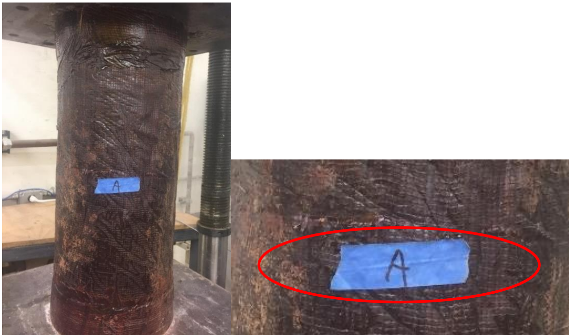
Figure 89. Typical compressive failure mode in the phenolic shell (Phenolic A)
