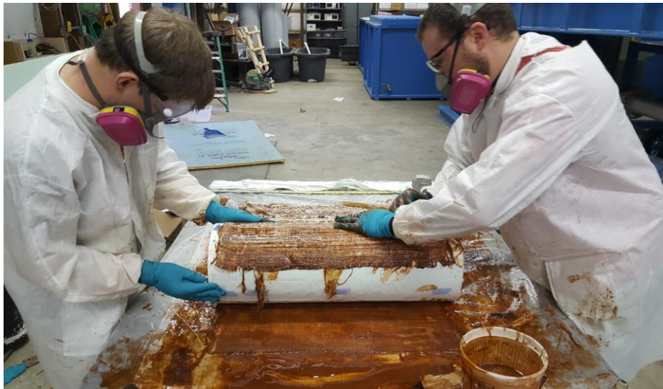
Figure 44. Wrapping of compression test tubes
