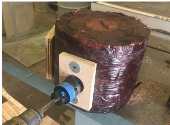
Figure 39. Cutting of timber for pull-off tests
