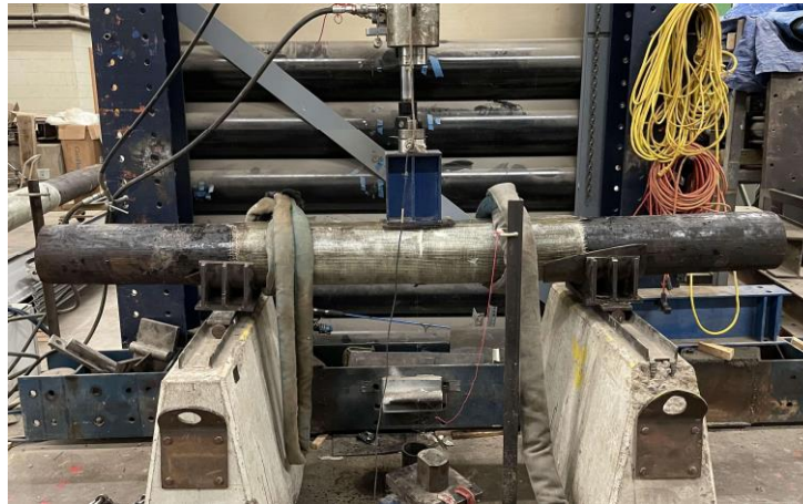
Figure A-2 – Six-layer FRP splice shear test
