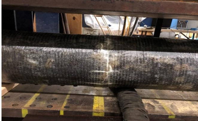
Figure 129. Bulging in FRP splice during compression testing
