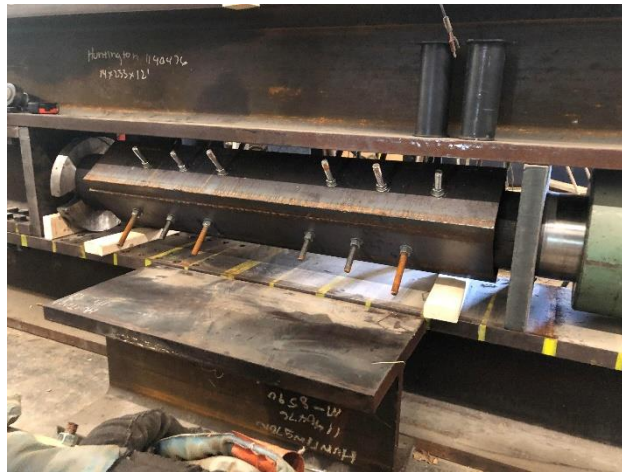
Figure 67. Axial test setup with C-channel splice
