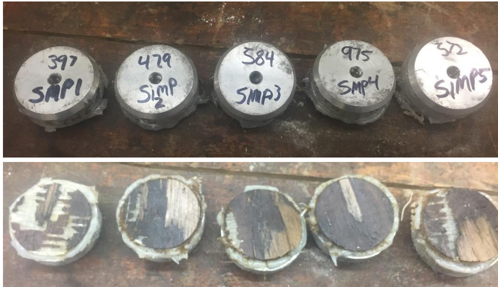
Figure 81. Simpson Strong-Tie pull-off carriers (timber failure)
