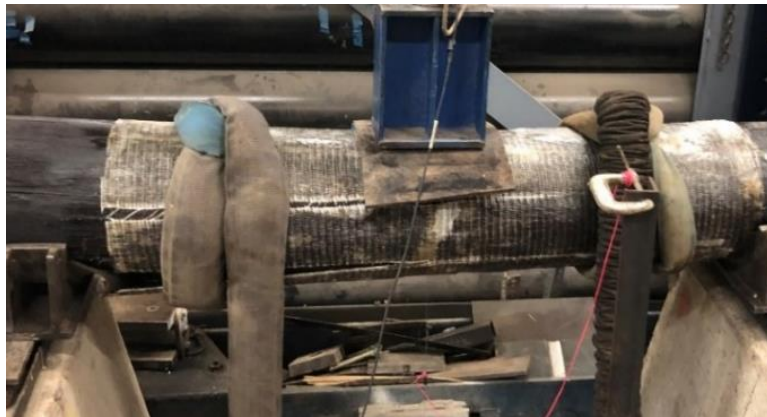
Figure 123. Hoop failure in shear test
