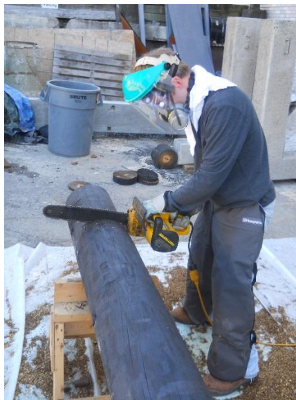
Figure 25. Cutting timber specimens
