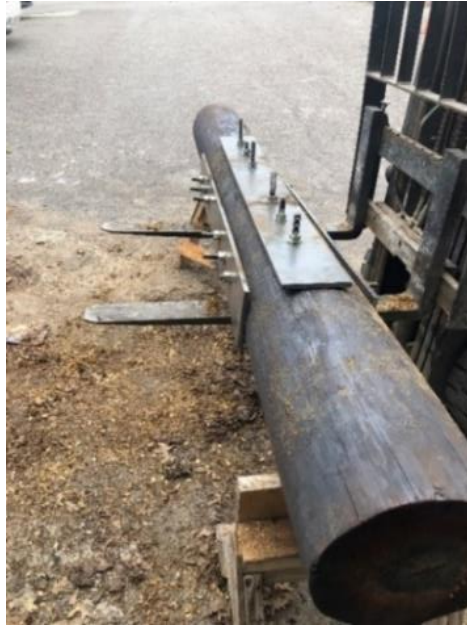
Figure 59. Steel splice specimen constructed in WVU CFC lab
