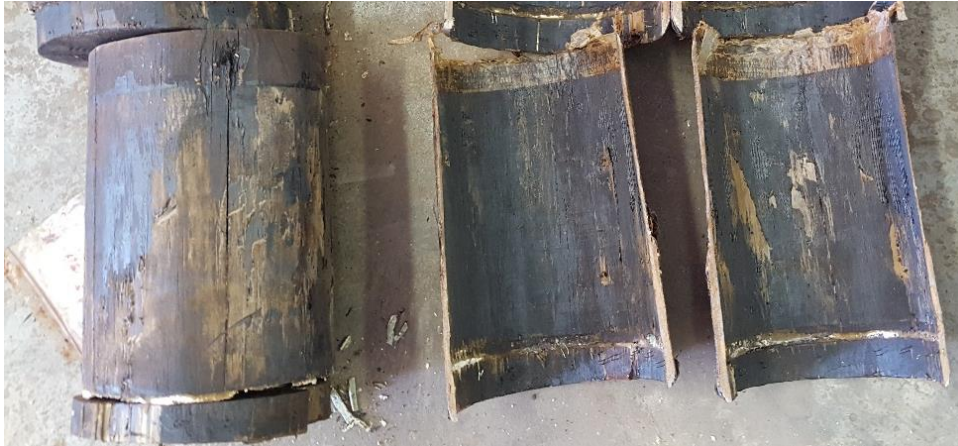
Figure 74. Superficial retained timber on phenolic wraps
