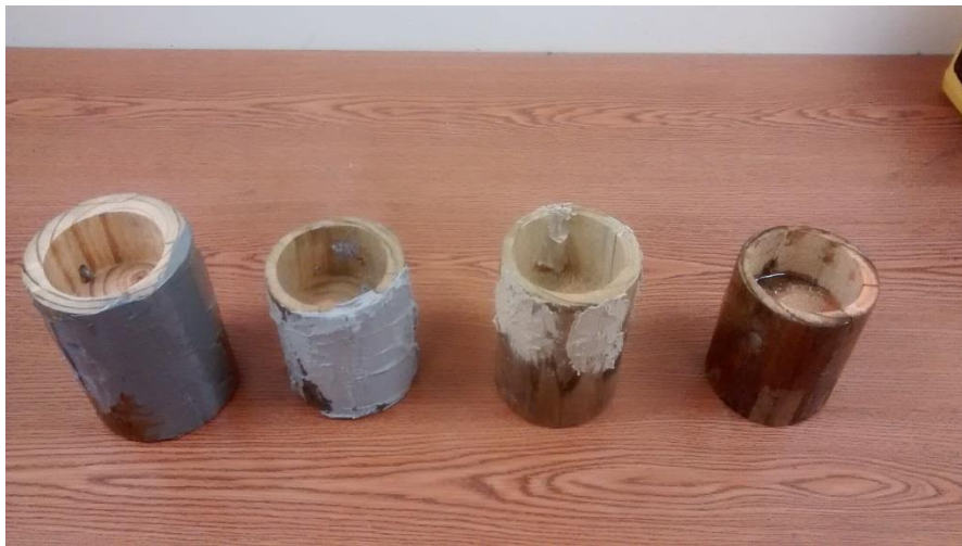
Figure 97. Prepared crack filler specimens
