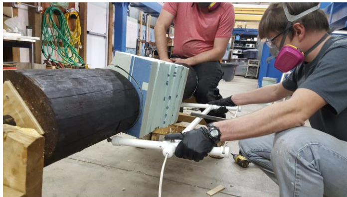
Figure 48. Trimming insulation for simulated rehabilitation
