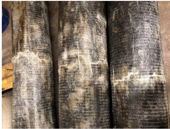
Figure 130. FRP splice axial compression specimen
