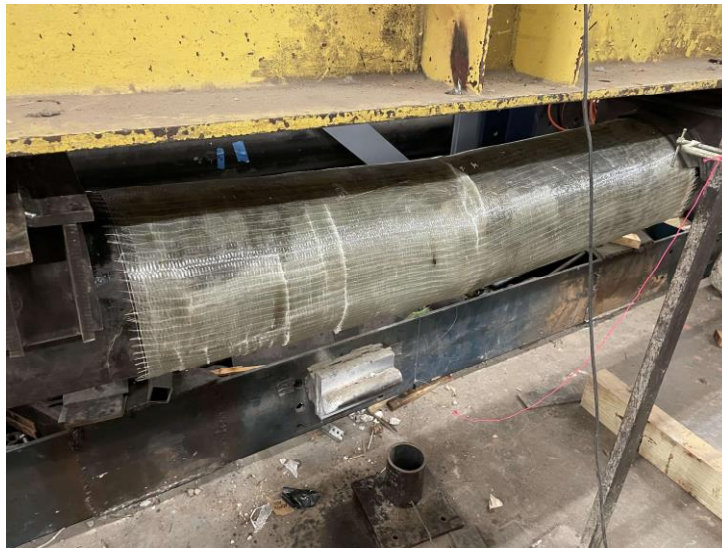
Figure A-6 – Splitting of fabric in re-wrap test
