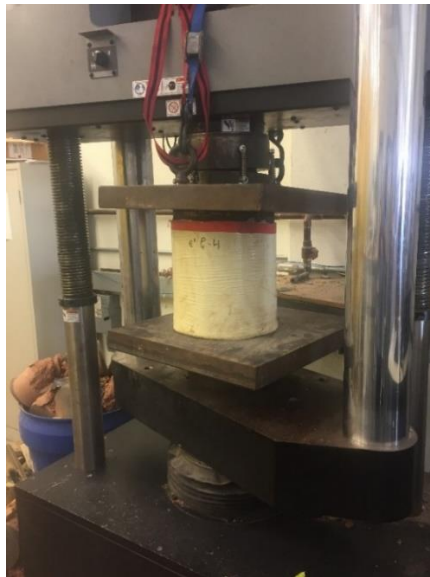
Figure 34. Testing configuration for bond test
