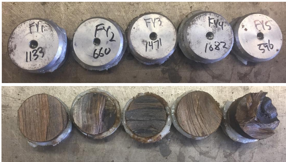
Figure 79. Fyfe pull-off carriers (timber failure)
