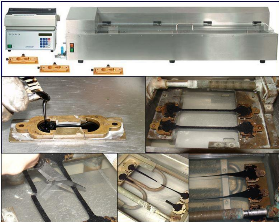
Figure 21 Typical ductilometer test setup
