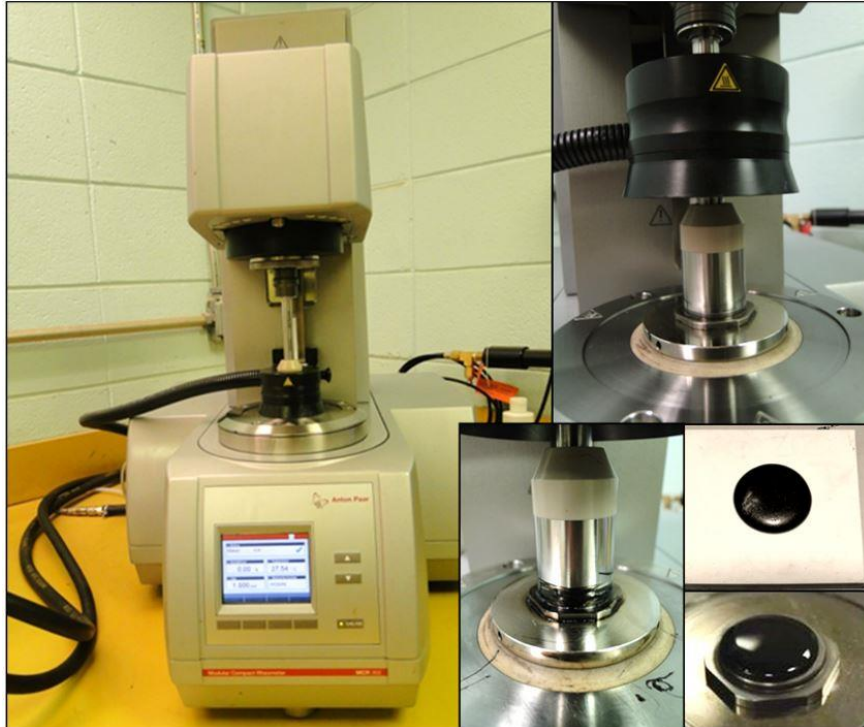
Figure 18 Anton Paar MCR 302 DSR
