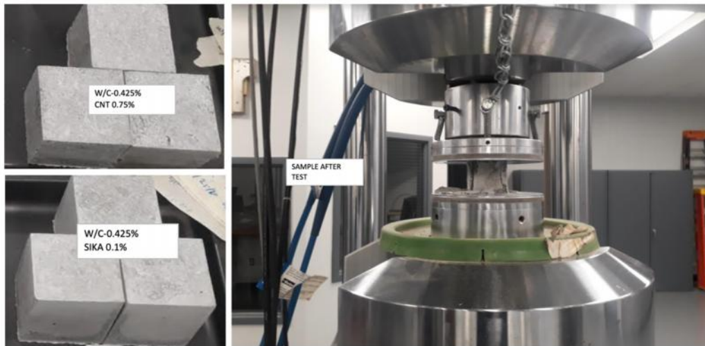
Figure 6: Compression Samples and Sample Testing in MTS
