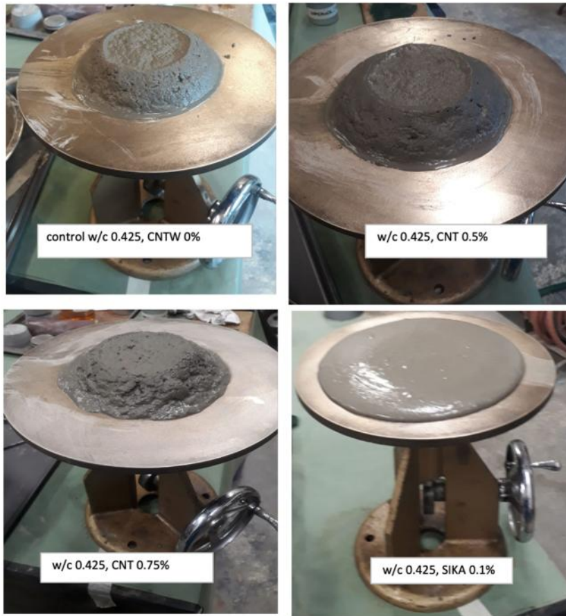
Figure 5: Mixture Condition After 25 Blow of Flow test
