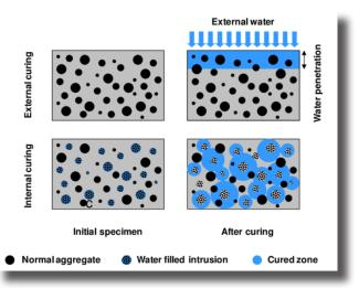
Figure 1. Differences between external curing and internal curing provided by pre-wetted LWAs
