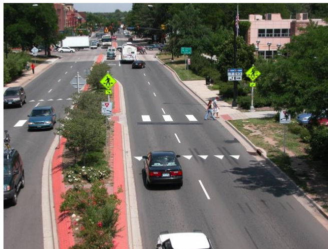
Figure B7. Advanced stop line
