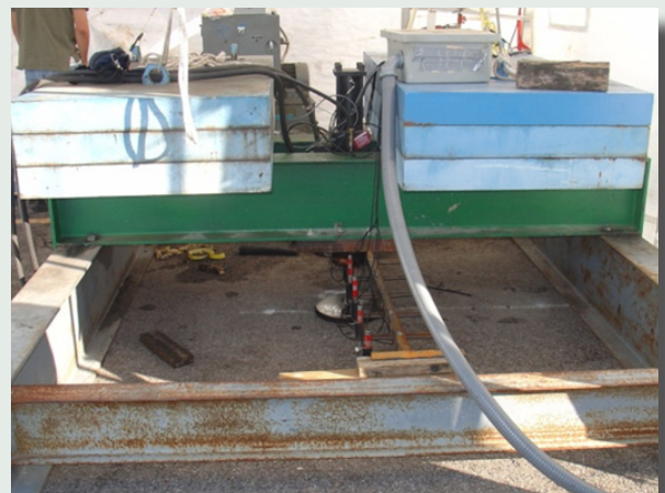
Figure 1 Outdoor setup of cyclic plate load test
