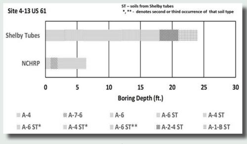
Figure 2 Soil strata from Shelby tube sampling and NCHRP soil unit data
