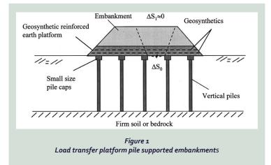
embankment on soft clay soil to improve the soil's ability to carry the applied load.
