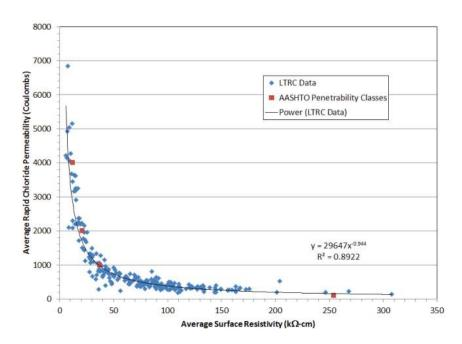
Figure 3. Relationship between surface resistivity and rapid chloride permeability at all ages for all samples tested [38]
