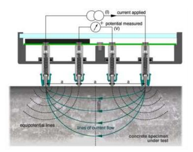
Figure 2. Schematic of the surface resistivity meter [36]
