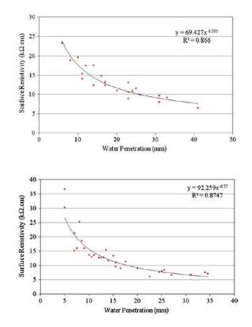
Figure 4. Relationship between EN 12390-8 water penetration and SR for plain mixtures (top) and for mixtures containing metakaolin (bottom) [46]
