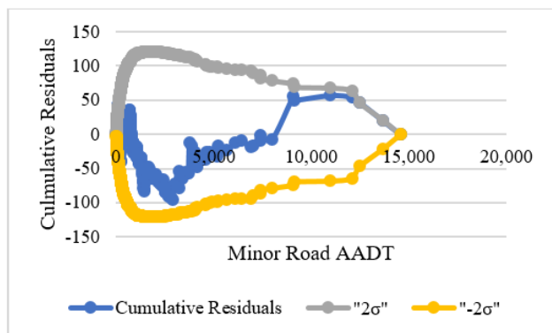
Figure 18. CURE plot minor road AADT vs. total crashes on urban two-lane three-leg intersections
