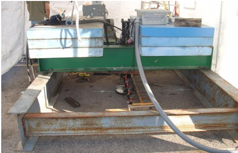
Figure 69. Outdoor setup of cyclic plate load testing facility
