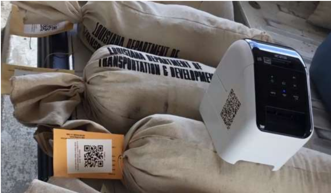
Figure 17. Picture of printer, samples, and corresponding QR codes for sample tracking in HeadLight
