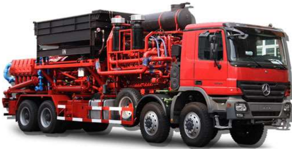
Figure 45 ACEWEL 2500 truck-mounted fracturing pump
