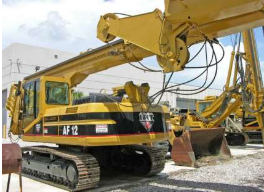
Figure 55 AF 12 drilling rig
