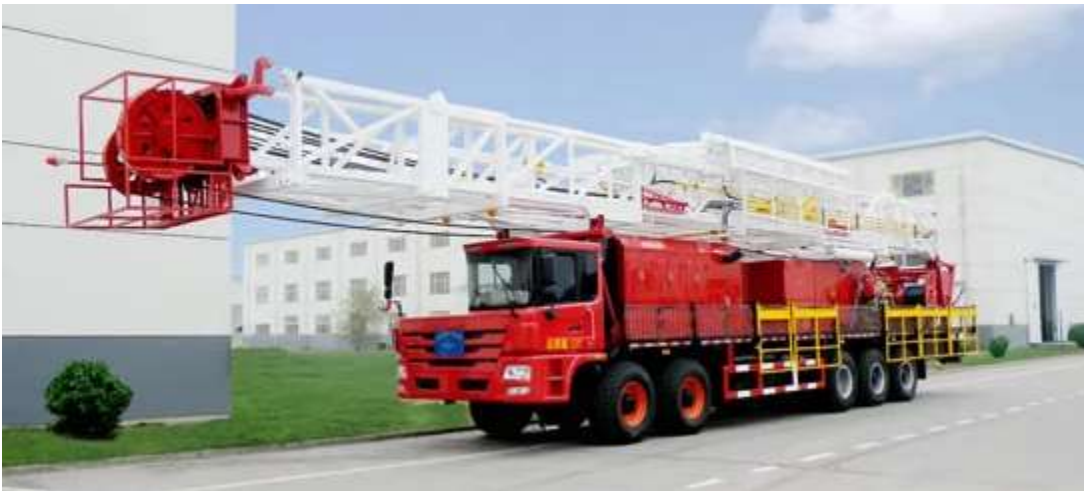
Figure 41 XJ 350 truck mounted workover rig
