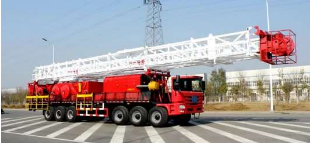
Figure 40 ZJ 10/900CZ truck mounted drilling rig
