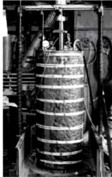
(b) Large-Size Triaxial Load Cell
