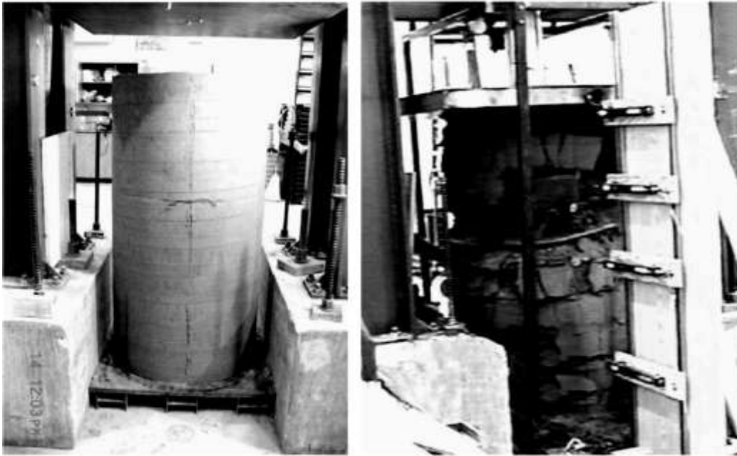
Figure 11 Cylindrical GRS setup before and during testing [57]
