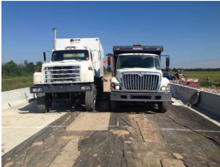
Figure 59 Static load test
