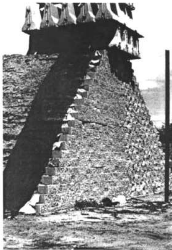
Figure 18 Loading test of the commerce city GRS wall [4]
