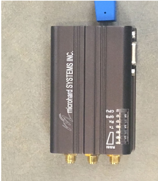
Figure 18 (a) Microhard Bullet-LTE cellular modem (b) antenna of cellular modem attached to cabinet
