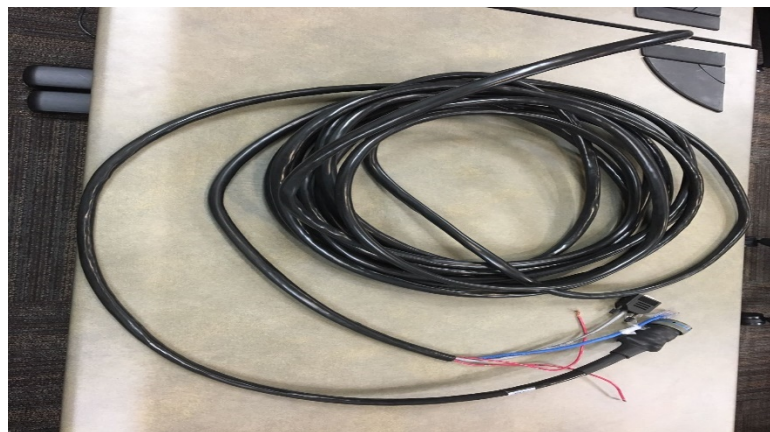
Figure 8 RTMS cable with communication and power outputs
