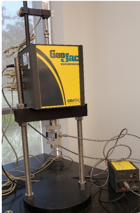
Figure 5. Unconfined compression test device.
