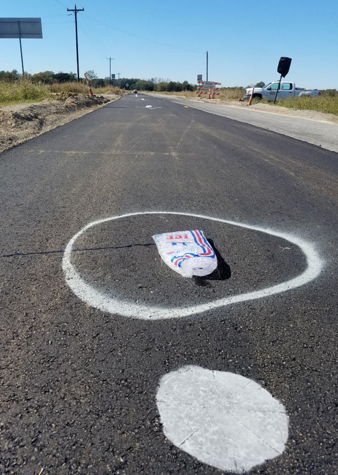
A typical test site. Coring either took place the day of paving or the next day. If coring was done on the same day, ice bags were laid on the spots to cool the spots before coring.
