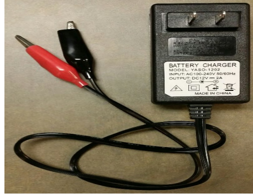
(f) Battery Charger
