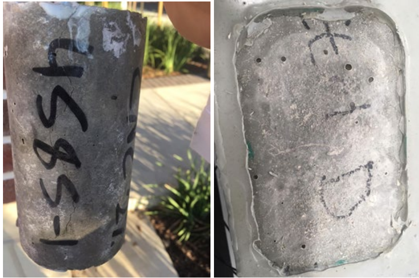
Figure 8. (a-left) crack sample cylinders, (b-right) crack beams samples.
