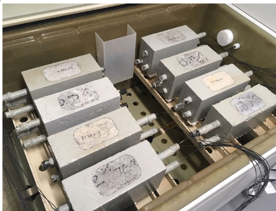
Figure 11. Three electrode system set-up for the fog chamber samples.
