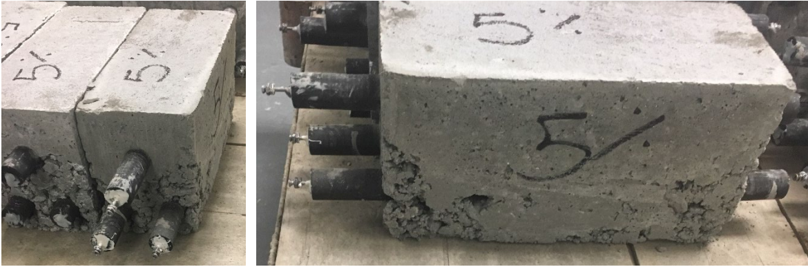
Figure 19. Honeycombing observed in TEA-C 5.0% specimens.
