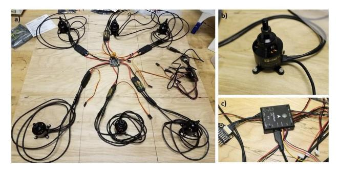
**Figure 5.** UAV electrical component wiring and integration activities. a) The six motors mounted to a benchtop integration setup along with electronic speed controllers and a power distribution board. b) A closeup of one of the six motors. c) The 3DR Pixhawk Mini flight controller, ready for programming via the USB uplink cable and associated laptop (not shown).
