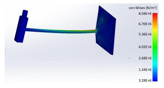
**Figure 3.** Finite element stress analysis of a single motor-arm-sidewall assembly in order to determine maximum stress magnitude and location.
