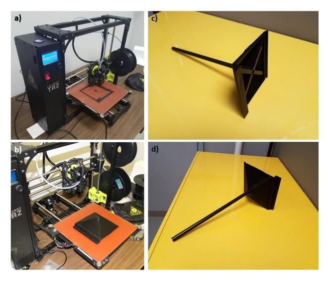
**Figure 4.** UAV body fabrication activities. a) A 3D print of one sidewall beginning. b) The completed sidewall. c) Inside view of the sidewall with graphite tube "arm" inserted. d) Outside view of the same sidewall/arm assembly.
