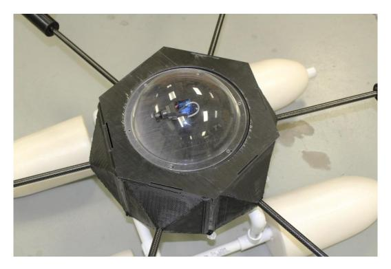
Figure 7. Close-up of the fully assembled UAV prototype hexcopter.
