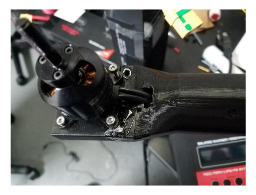
Figure 8. Close-up of the broken motor mount after a repair attempt was made. Fracture was across the two bolts holes on the right.
