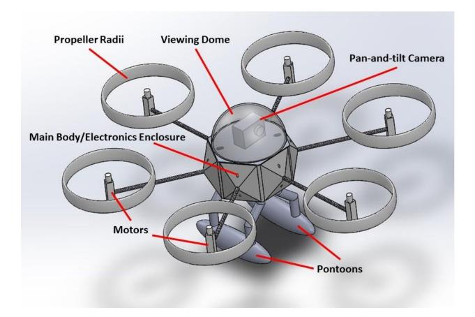
Figure 2. Annotated computer model of the assembled inspection drone.
