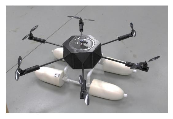
Figure 6. The fully assembled UAV prototype hexcopter.
