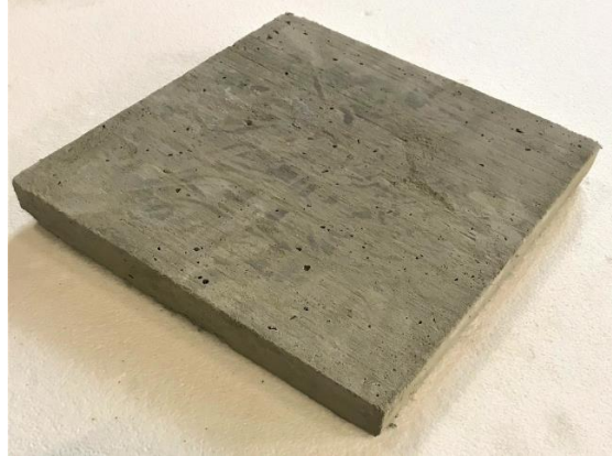
Figure 2 ECC panel sample for impact test
