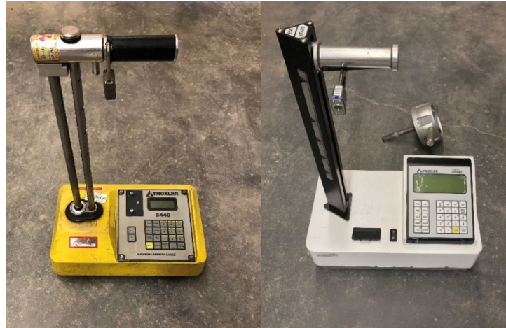
Figure 3 Soil density gauges (NDG on left; LNDG on right)
