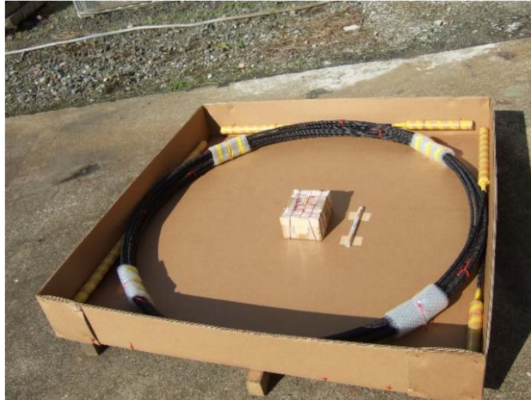
Figure 3(b) Carbon fiber composite cable
