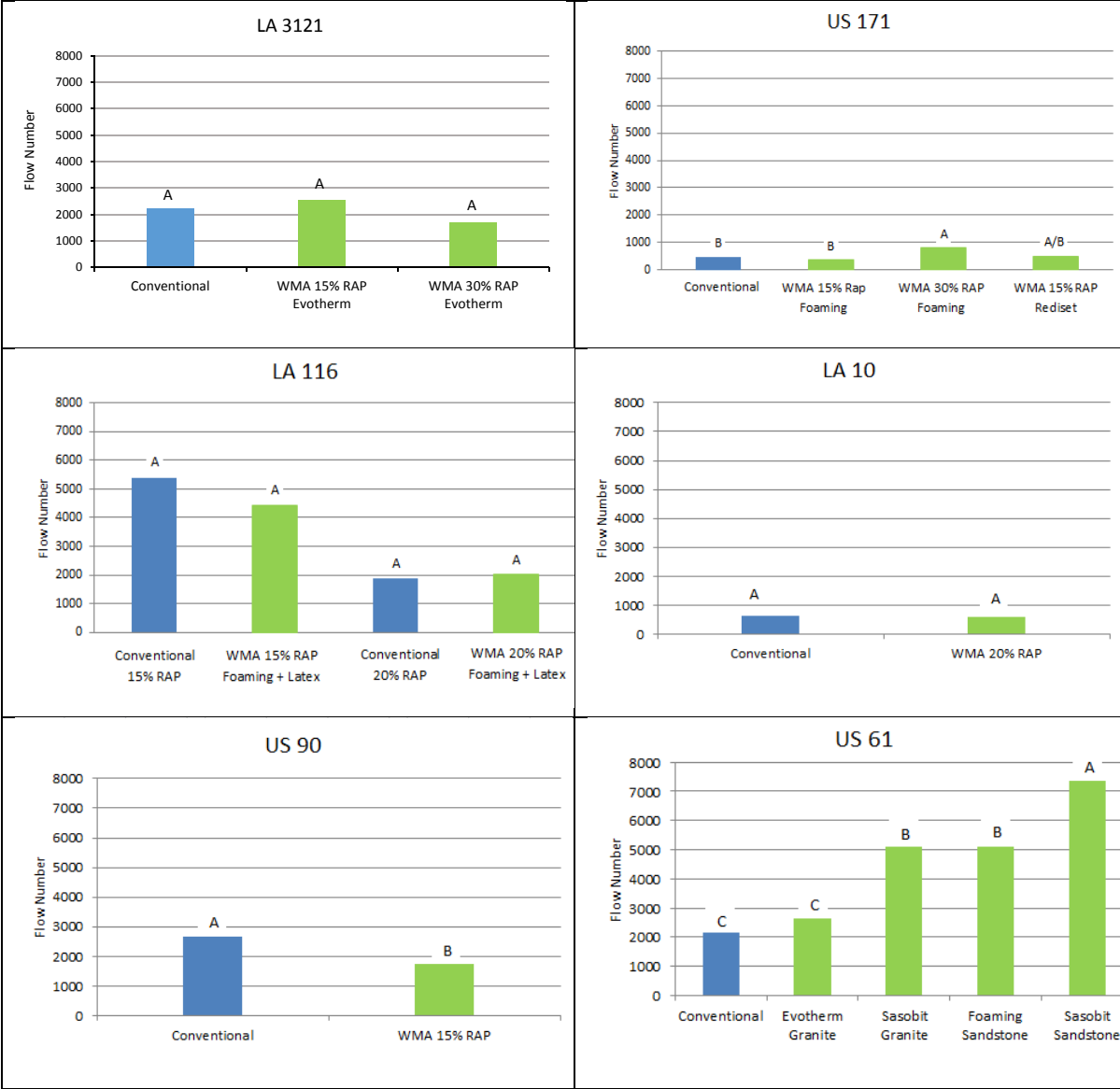
Figure 93 Statistical analysis of flow number results
