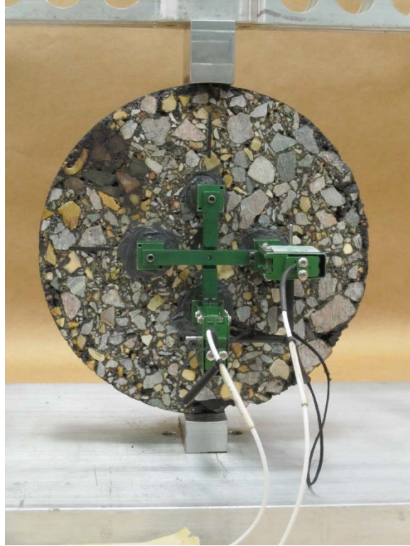
Figure 114 Specimen instrumented for the DCSE test
