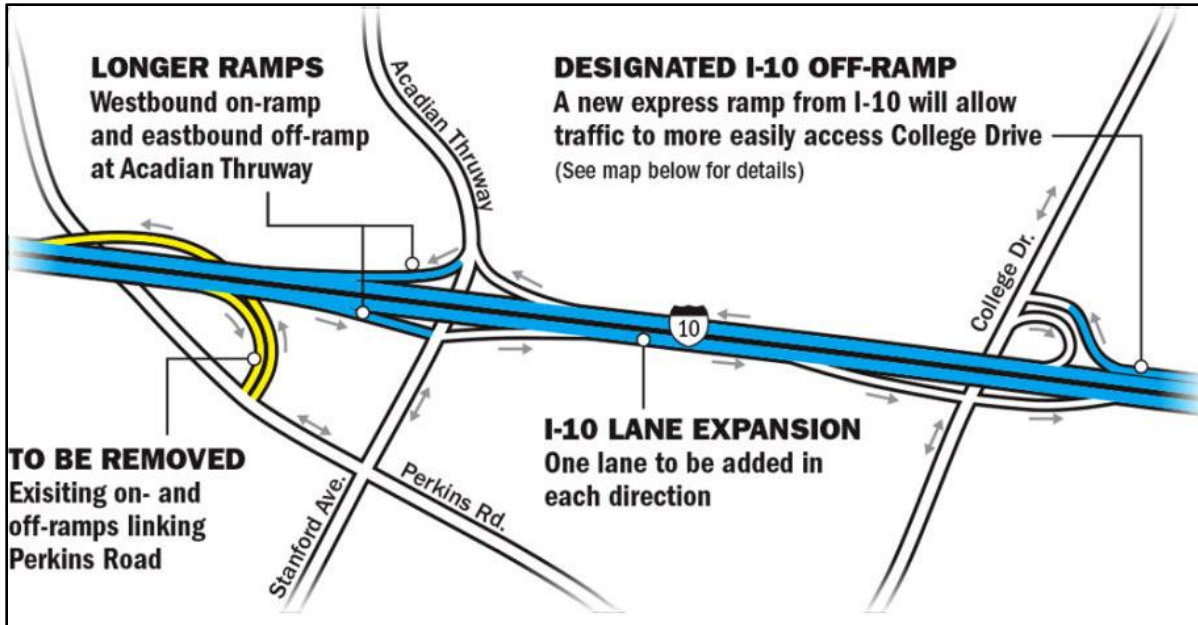
Figure 5. Stage-2: Redesign and reconstruction of exits and ramps at Perkins Road, Acadian Thruway, and College Drive (17).
