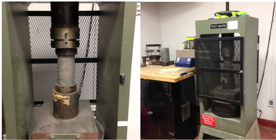
Figure 6: Testing of concrete cylinders
