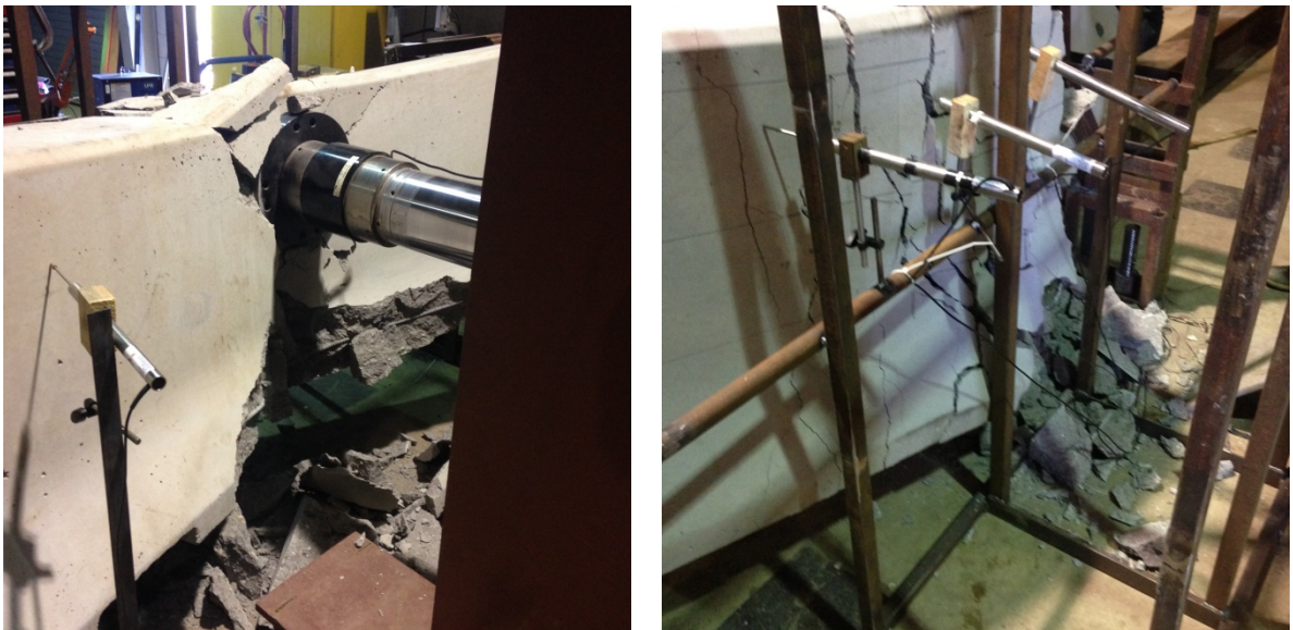
Figure 23: Failure of the barrier at 34.85 kip, displacement 1.51 in.
