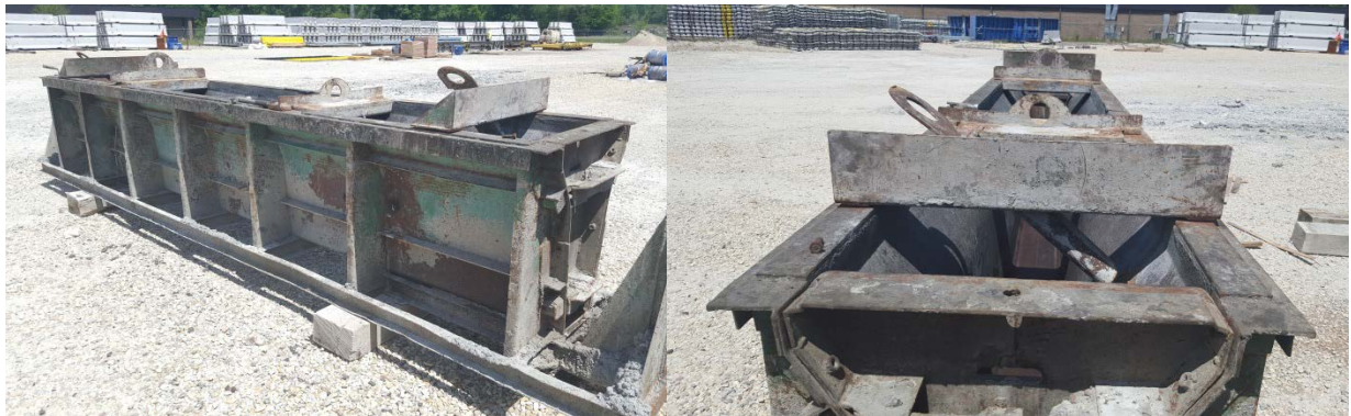
Figure 8: Steel form at the Waskey facility in Baton Rouge, LA
