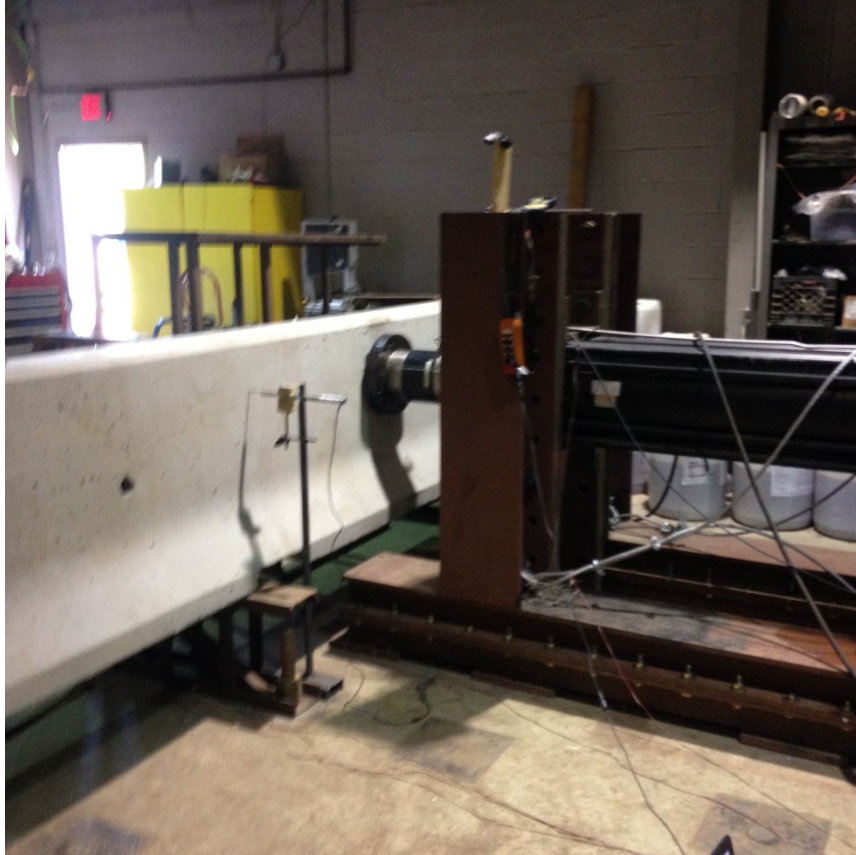
Figure 22: Actuator applying the bending load and instrumentation on the bending side
