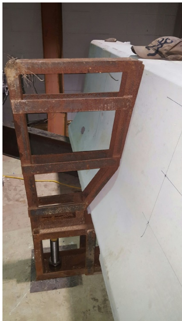
Figure 21: Positioning the barrier on the frame and instrumentation setup on the tensile side
