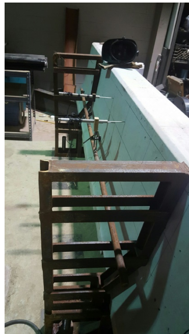
Figure 21: Positioning the barrier on the frame and instrumentation setup on the tensile side
