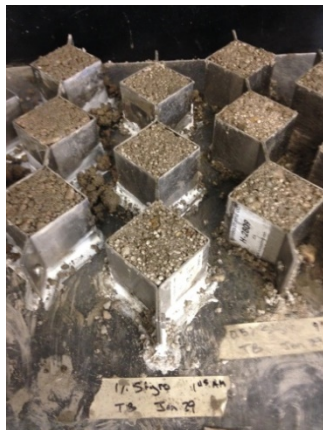
Figure 2: Cubes made with Styrofoam (left) and Tire dust (right)
