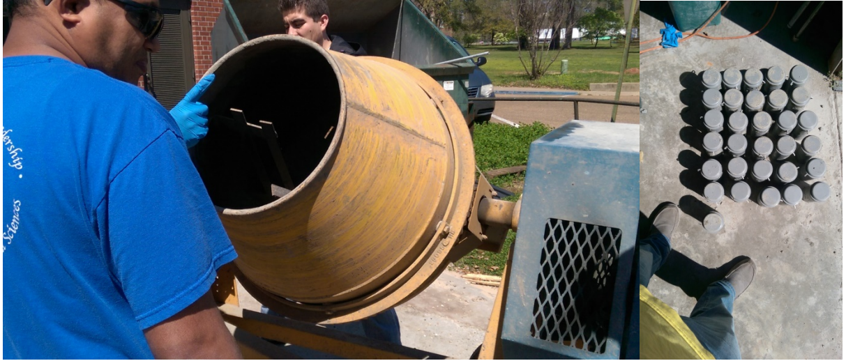
Figure 5: Preparation of sample mix designs and making of cylinders
