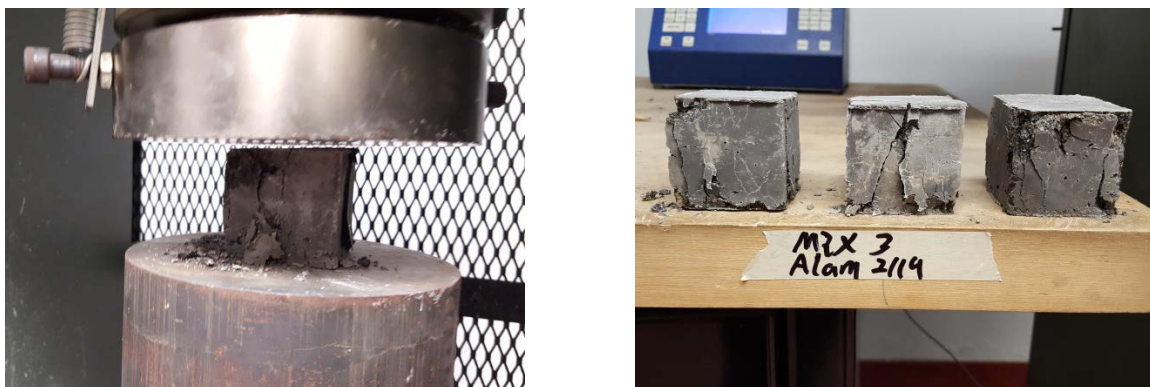
Figure 4: Testing of the cubes after 7-days of water curing
