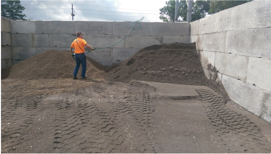
Figure 7: Watering of the aggregates at the Waskey facility in Baton Rouge, LA
