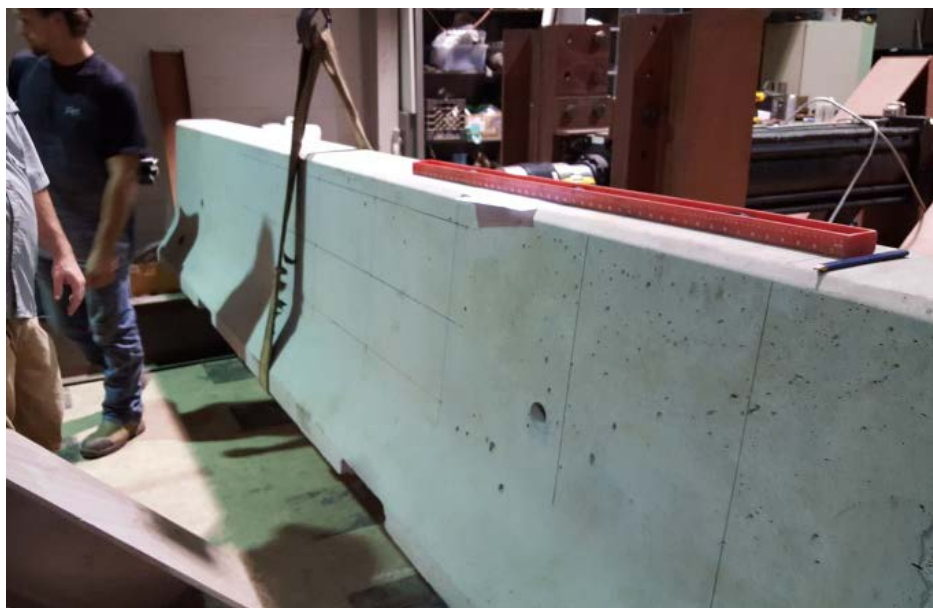
Figure 16: Positioning the barrier for testing
