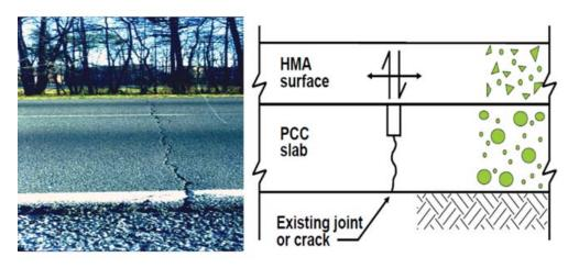
Figure 1 Reflective cracking
