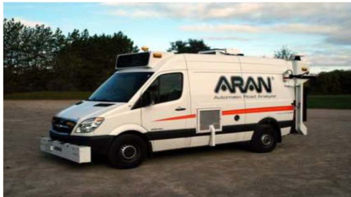
Figure 3 ARAN vehicle used by LA PMS
