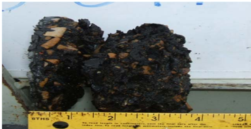
Figure 29 Example of severe stripping in control section 161-08
