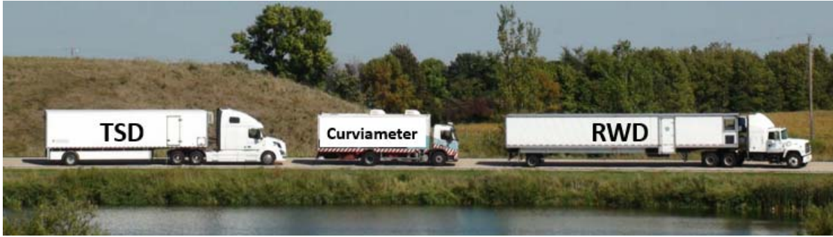
Figure 24 MnROAD continuous deflection testing program [33]
