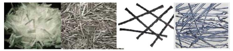
Figure 1 Polypropylene fibrillated fiber (left), polypropylene macro fiber (left middle), carbon fiber (right middle) and steel fiber (right)
