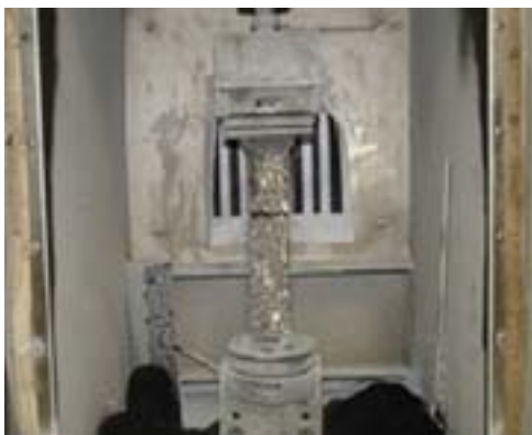
Figure 4 The thermal stress restrained specimen test
