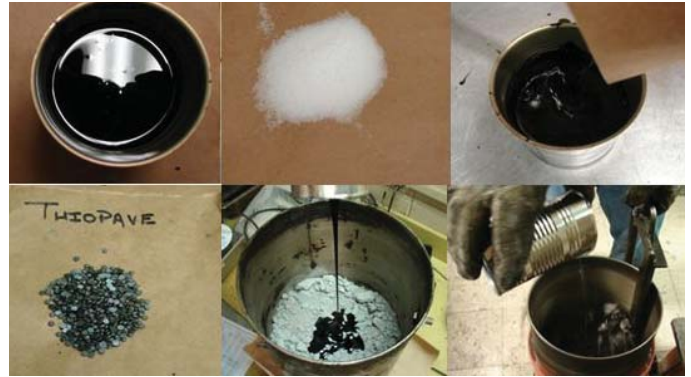
Figure 1 Illustration of the laboratory preparation of sulfur-modified asphalt mixture materials
