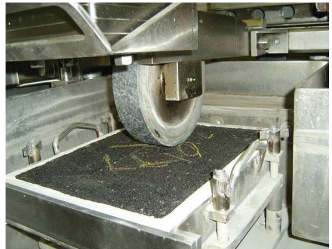
Figure 2 The Hamburg-type loaded wheel tester
