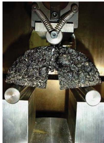
Figure 3 The semi-circular bending test
