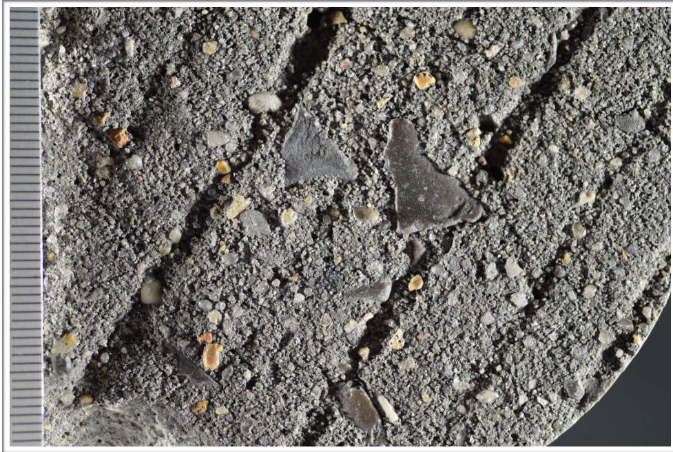
Figure F3. Photograph showing detail of the top surface of the core; scale in millimeters.
