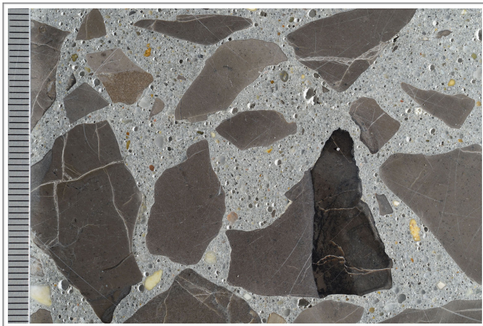
Figure I13. Photographs showing overview of polished surface in the middle of Core P#2; scale in millimeters.
