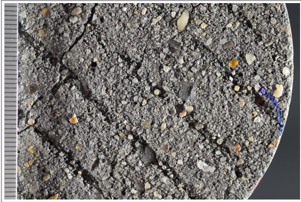
Figure G3. Photograph showing detail of the top surface of the core; scale in millimeters.
