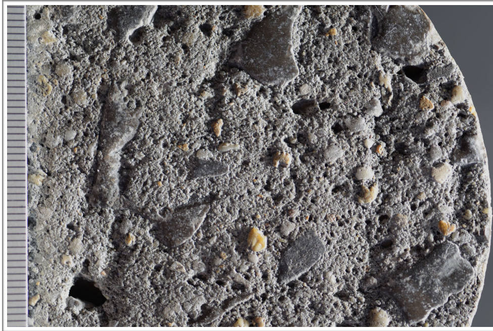
Figure A3. Photograph showing detail of the top surface of the core; scale in millimeters.
