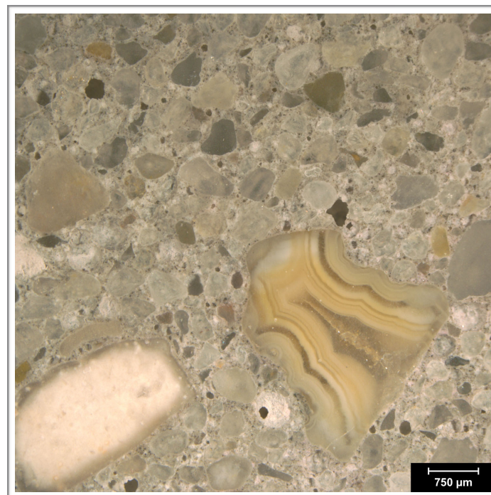
Figure A9. Reflected light photomicrograph of polished surface showing the fine aggregate.
