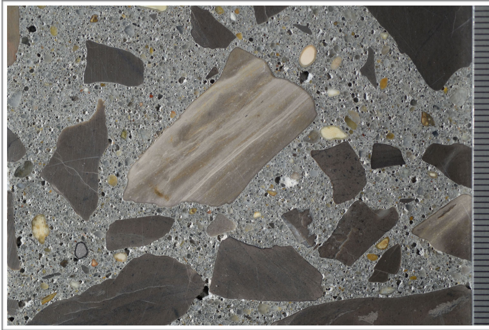
Figure B7. Photograph of the polished surface showing coarse aggregate; scale in millimeters.
