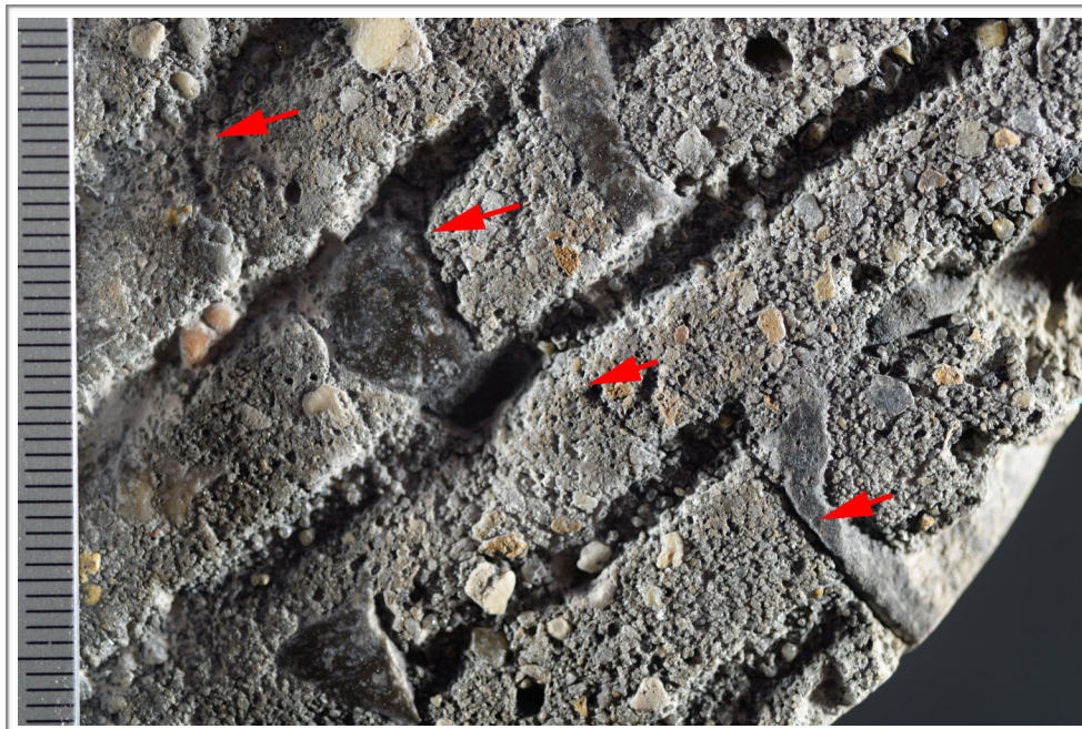
Figure B4. Photograph showing crack (red arrows) on the top surface; scale in millimeters.
