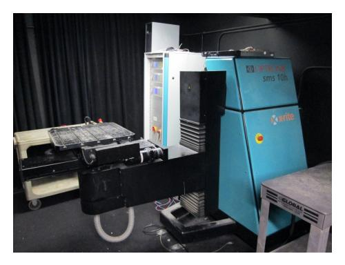
Figure 10 Goniometer to position the LED signal module according to each one of the angle coordinates from ITE (source: Intertek)
