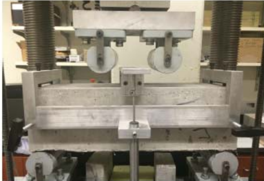
Figure 17 Side view of testing rig for ASTM C1609
