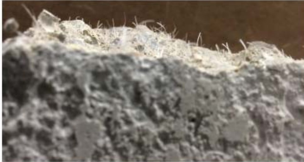
Figure 20 Broken section of polypropylene fibrillated fiber reinforced sample showing the length of the fibers reaching across the crack
