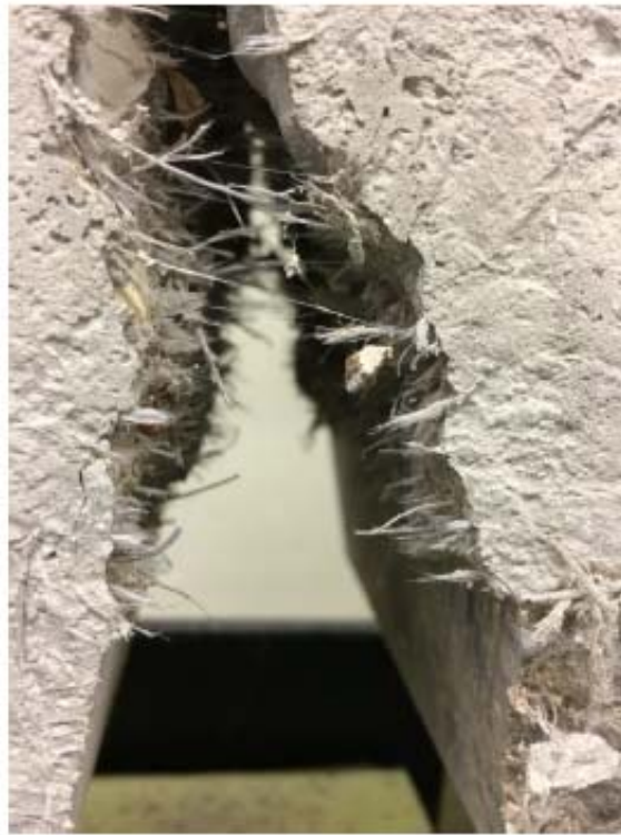
Figure 31 Failed pre-cracked sample showing broken fibers
