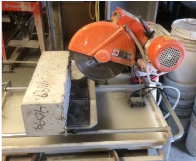
Figure 9 Wet saw setup for notching beams
