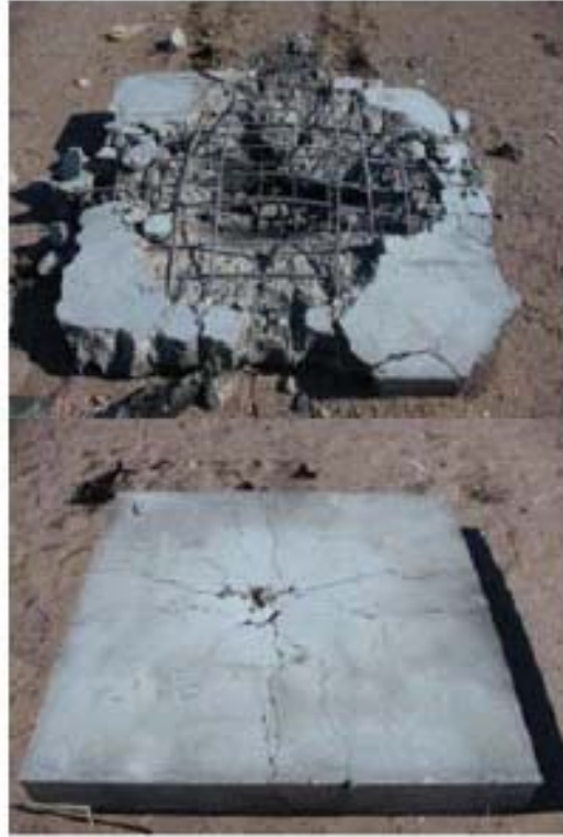
Figure 5 Comparison of traditional reinforced concrete (top) and fiber reinforced concrete (bottom) to blast [24]
