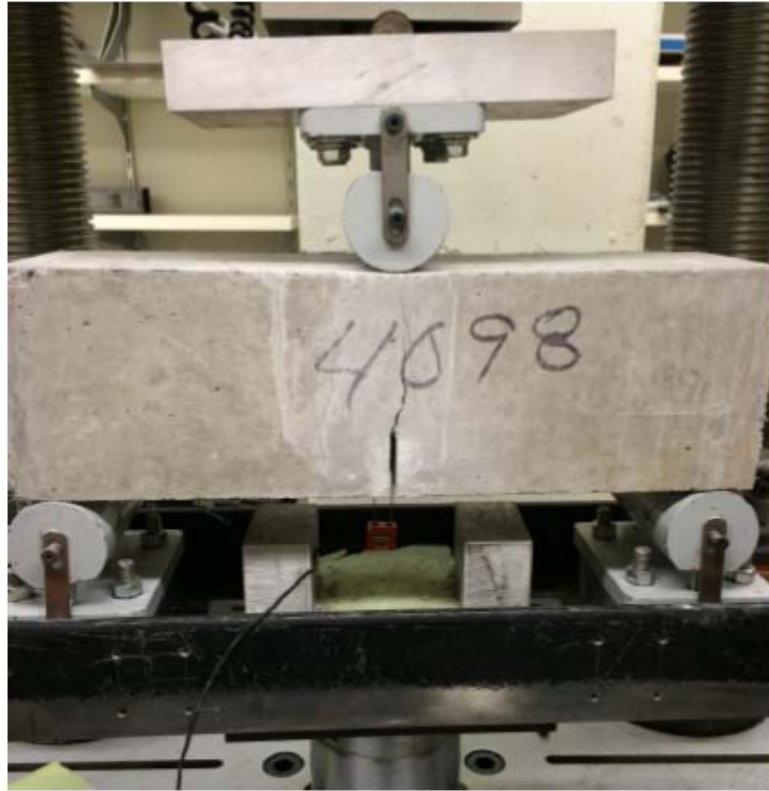
Figure 13 Notched beam testing after failure
