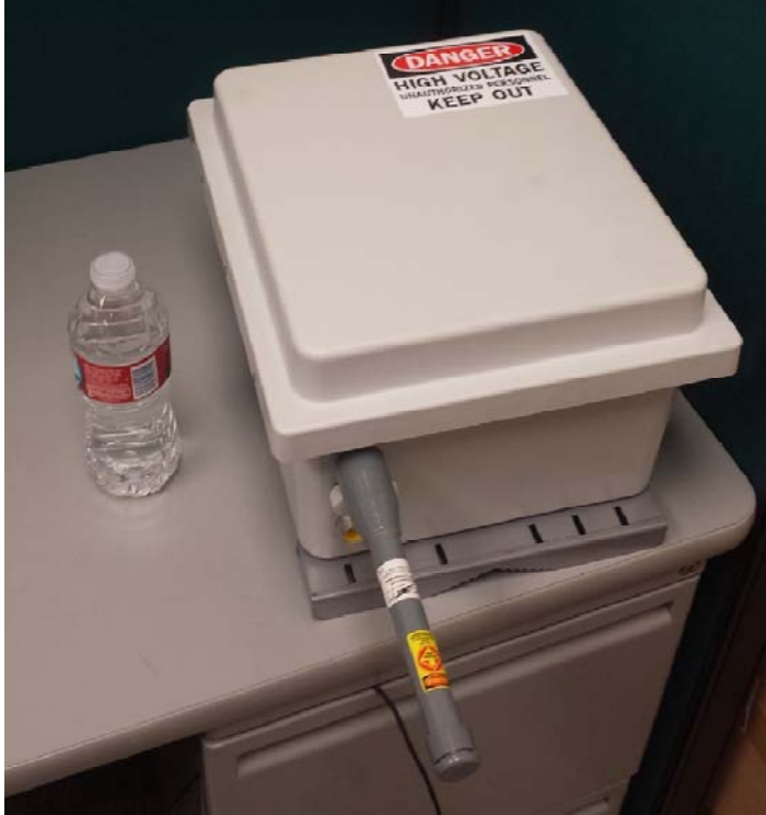
Figure 6 Bluetooth probe detection system cabinet
