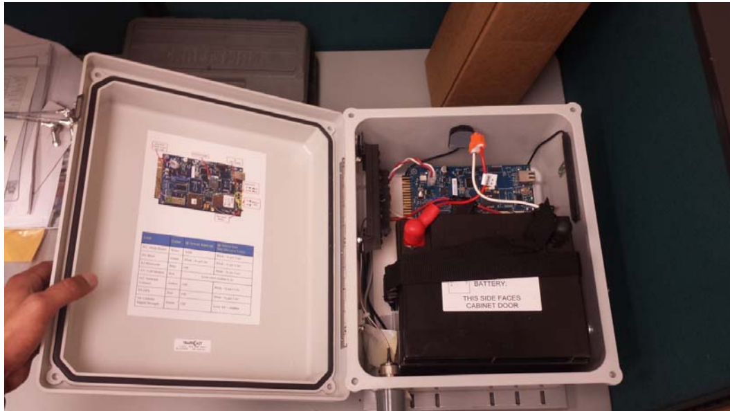
Figure 7 Components of Bluetooth probe detection system
