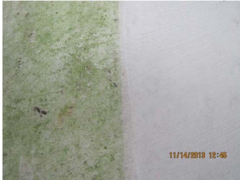
Figure 34 Self-cleaning property: close-up of coated (on right) and non-coated (on left) surface highlights self-cleaning
