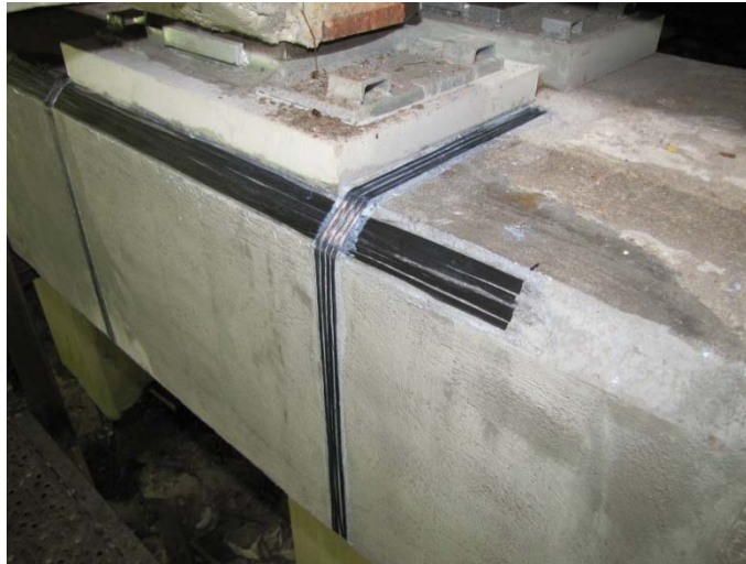
Figure 18 Detail of horizontal and vertical tows junction
