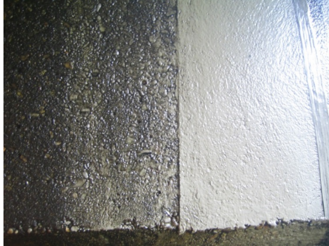
Figure 39 Self-cleaning property: Close-up of coated (on right) and non-coated (on left) surface highlights self-cleaning
