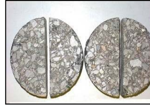
Step 2: Cut specimens along the center diameter
