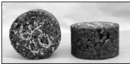
Step 1: Prepare gyrotory-compacted samples
