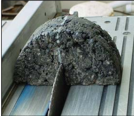
Step 3: Create notch with desired depth
