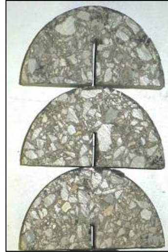
Step 4: Repeat procedure for three notch depths
