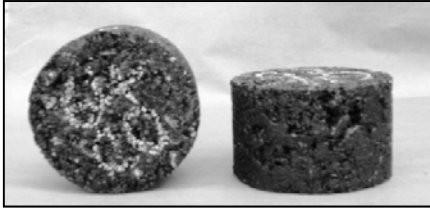
Step 1: Prepare gyratory-compacted samples
