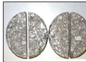
Step 2: Cut specimens along the center diameter
