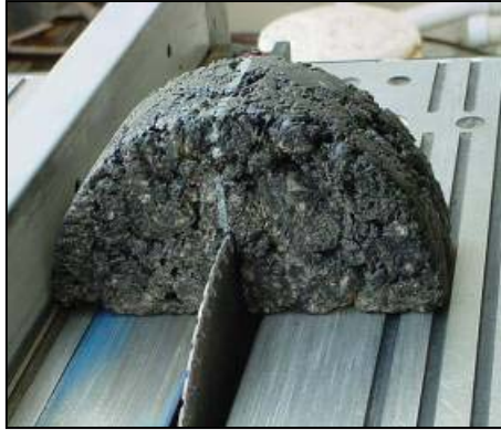
Step 3: Create notch with desired depth
