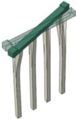
Figure 85 Torsion applied around Z direction; (a) Deformed and undeformed meshes of the pile group; (b) moment-rotation curve
