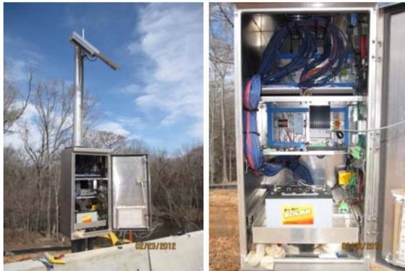
Figure 33 Data acquisition system including solar panel
