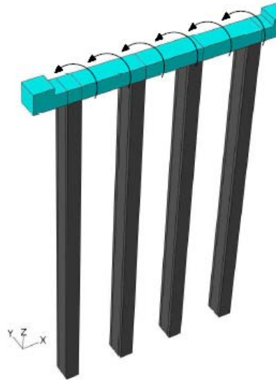
Figure 75 Moment applied to the top of the bent around the X direction
