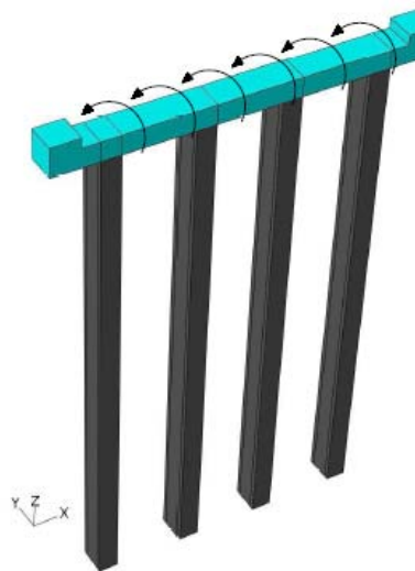
Figure 60 Moment applied to the top of the bent around the X direction
