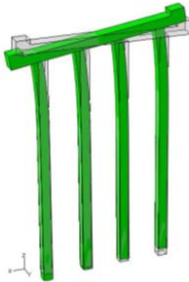
Figure 73 Deformed and undeformed meshes of the pile group due to a moment around the Y direction.
