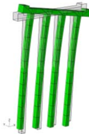
Figure 58 Deformed and undeformed meshes of the pile group due to a moment around the Y direction
