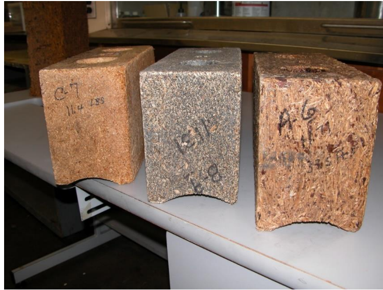
Figure 8A Guardrail block (side view)
