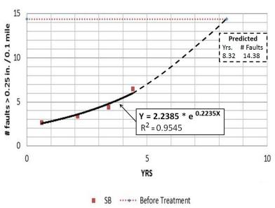
Figure 14 Faulting vs. years (southbound roadway)
