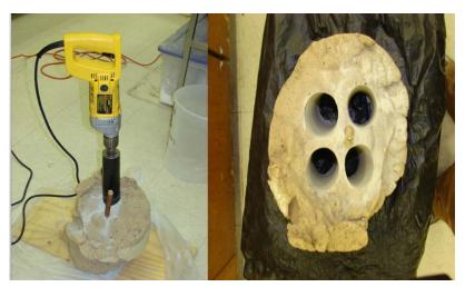
Figure 36 Coring sand/PF bucket sample
