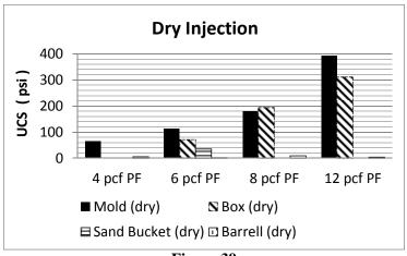
Figure 39 UCS dry injection sample comparison
