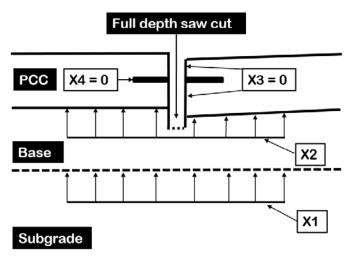
Figure 7 Joint with full depth saw cut
