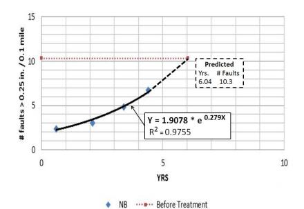
Figure 13 Faulting vs. years for northbound roadway
