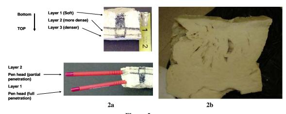
Figure 2 Polyurethane heterogeneous samples
