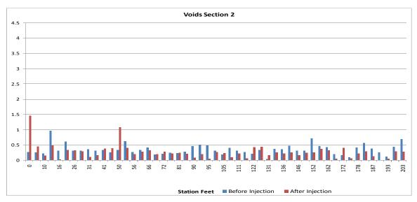
Figure 16 Void potential for test section 2
