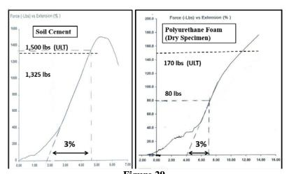
Figure 29 Load versus extension graphs
