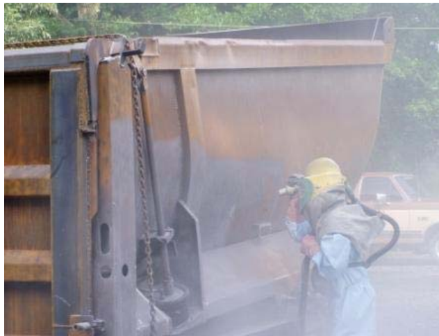
Figure 18 Soda blasting of a steel container prior to repainting [37]
