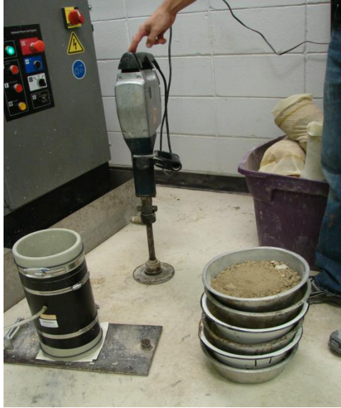
(a) Vibratory Compacter and Mold
